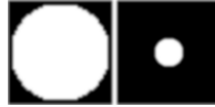
Fig. 4 Patch containing the disk (left) is inserted into a black background to create a noise-free frame of the movie (right).
