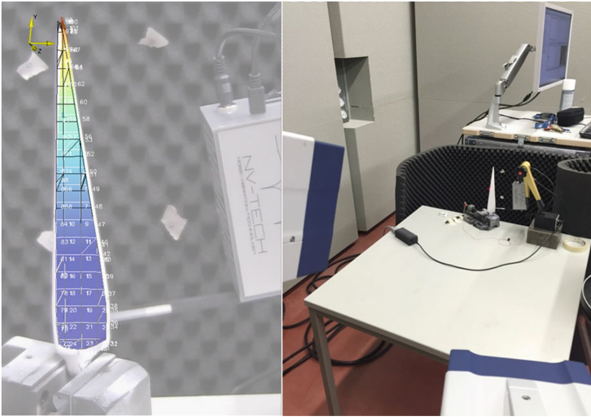
Fig. 2.4 Left —Clamping of the propeller blade and SAM impact position. 101 DOFs were used for this modal analysis. Right —Experimental setup for this test. A large angle between scanning laser heads was needed in order to better acquire the in-plane vibration components
