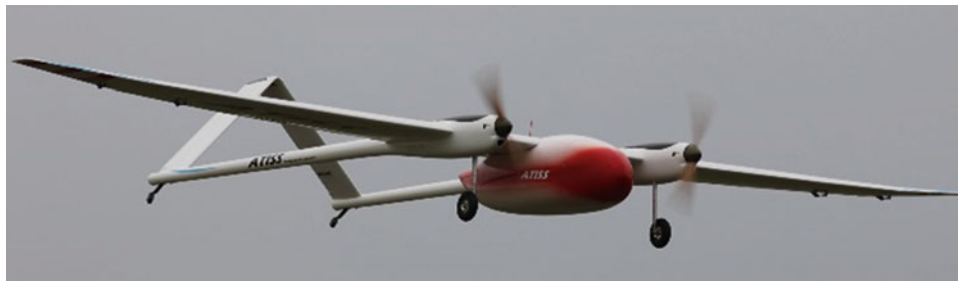
Fig. 2.1 The ATISS drone with the red painted payload container between the rotors. It has a wingspan of about 5 m and an empty weight of 15 kg
