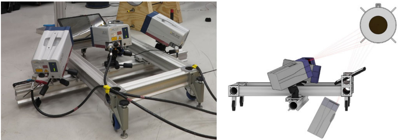
Fig. 1.8 Photograph ( left ) and schematic ( right ) of the laser cart used to scan the bottom quadrants of the empty bomb case. The schematic shows the effective position of the mirrored laser head
