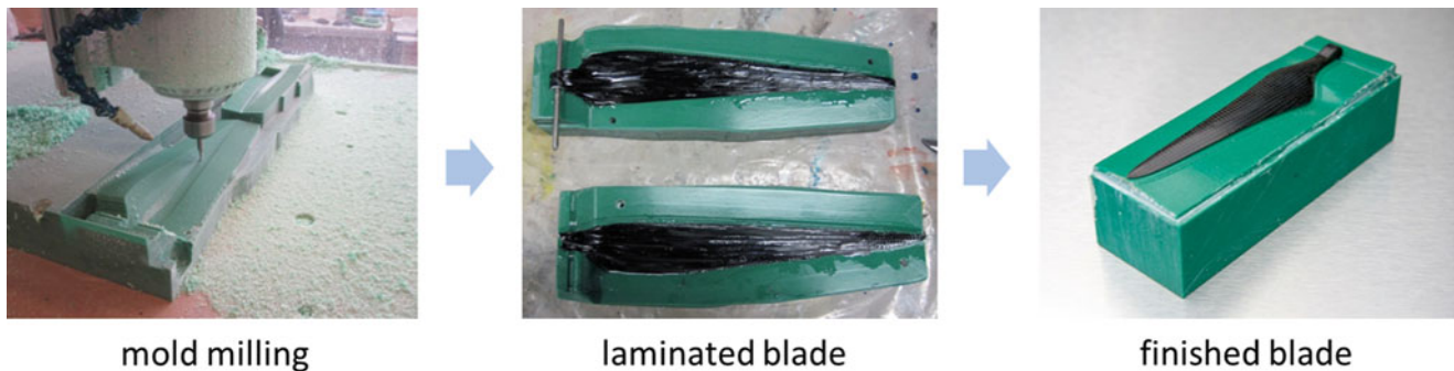
Fig. 2.2 Manufacturing process of the propeller blade used on this study
