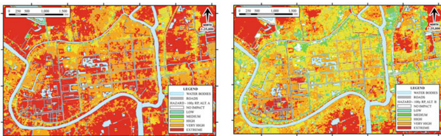
Fig. 29.6 Example of hazard assessment (existing situation—left, and incorporation of new flood protection measures—right); The hazards were substantially reduced with the proposed measures
