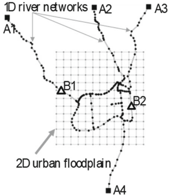
Fig. 29.3 Modelling framework: 1D-2D model where 1D is used for the river network and 2D for the terrain in the Ayutthaya Island
