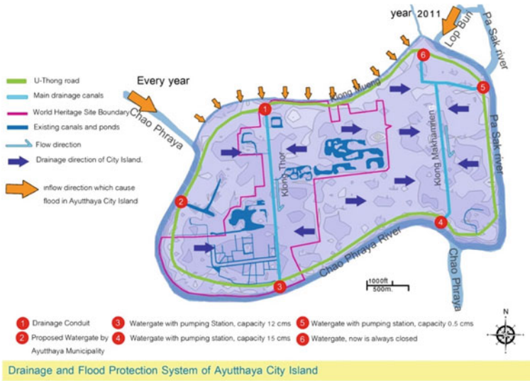
Fig. 29.7 Illustration of the key drainage and flood protection measures in the Ayutthaya heritage area
