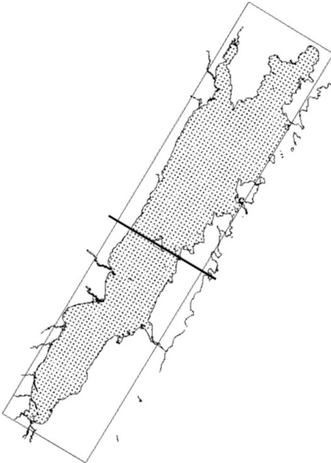
Fig. 2.2 Sketch of the grid used for the nested grid model. The model obtains boundary conditions at the mouth region between Green Bay and Lake Michigan from the GLCFS model, and tributary inflows from USGS Web sites. The dark line across Chambers Island delineates the grid used for Lower Green Bay model simulations
