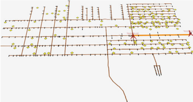
Fig. 4 Power distribution networks of micropolis: the red towers are the power substations; the light orange line is the MV distribution line; brown lines are the distribution feeders; and yellow diamonds are the PV systems installed (Color figure online)
