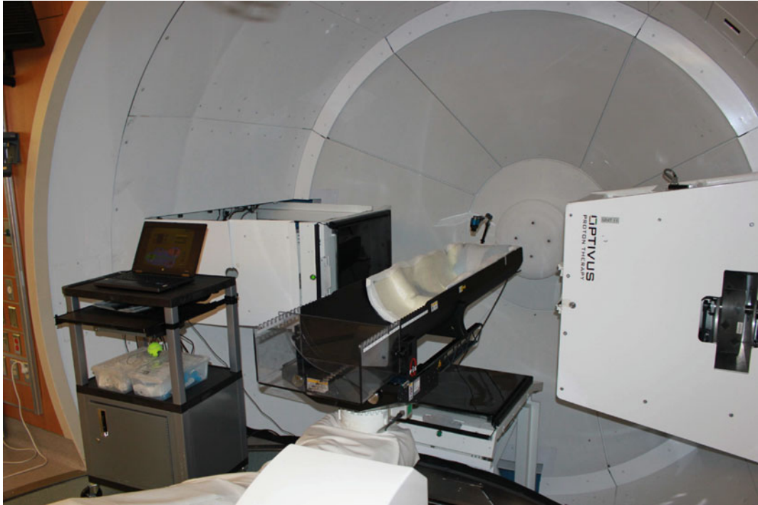
Fig. 10.3 Patient setup at Loma Linda utilizing pod immobilization and SDX for active breath management for treatment of liver tumors
