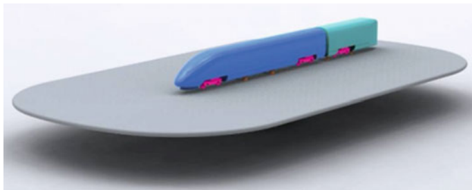
Fig. 14.1 NGT2 front car model with streamlined end body attached to a stationary flat plate as used in the experiment
