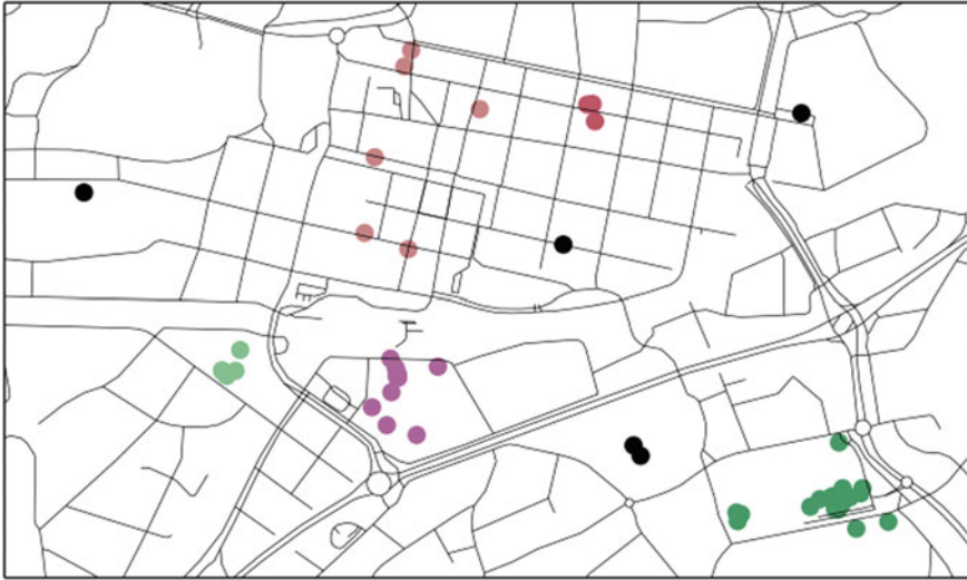
Fig. 7.2 DBSCAN \epsilon = 200 m. Points with similar color are categorized into one cluster where noise points are depicted in black . By increasing the \epsilon value from 100 to 200, compared to Fig. 7.1, the points in the parking lot are clustered together, while many of the noise points (corresponding to distinct destination) in the city center are merged into one large cluster
