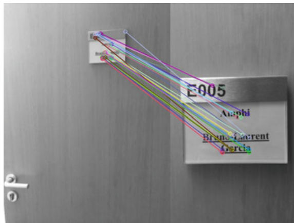
Fig. 5 Doorplate detection using the ORB feature detector running on a Raspberry Pi B board
