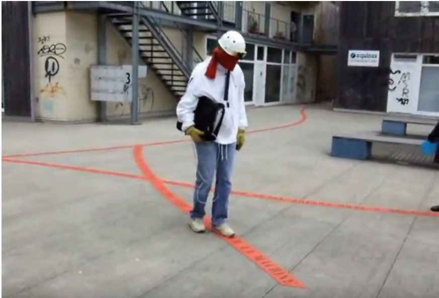
Fig. 8 A blindfolded subject equipped with the See CoLoR device composed of a stereoscopic pair of cameras and a stereo headset. Information from the cameras are processed by a laptop which delivers the sound signal allowing the subject to follow a colored ( red ) path. From Bologna et al.
