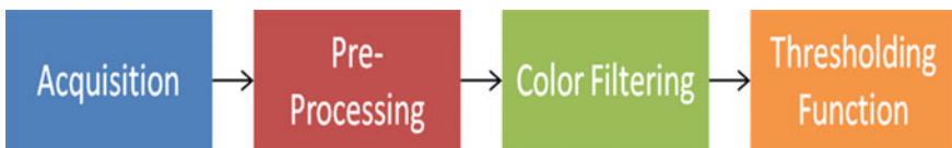
Fig. 3 Main step of the image processing on the smartphone for traffic light status discovery
