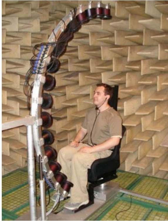
Fig. 9 Equipment for fast measurement of individual HRTFs
