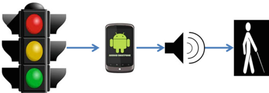
Fig. 2 Block diagram of the system for traffic light status communication to a VIP
