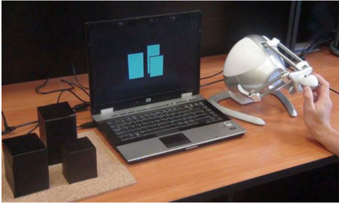
Fig. 15 A haptic interface bench. From left to right: model cardboard scene, 3D computer model of the scene, haptic interface programmed to simulate the virtual scene
