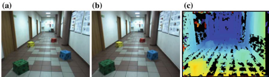
Fig. 6 Three-dimensional reconstruction of the “corridor” scene from stereovision: a left (reference) image, b right image, c depth map is pseudo-colors (the color palette codes the depth of the scene objects ; warm colors represent objects in close proximity whereas cool colors represent distant objects)
