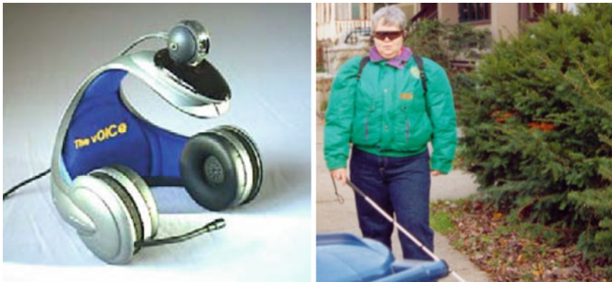
Fig. 6 The vOICe system from Meijer et al. The system is composed of a stereo headset and a head worn camera. Right individual using a portable version of the device while walking on a street
