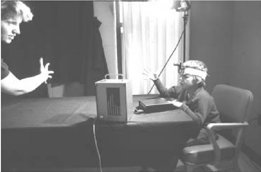
Fig. 1 Young subject reproducing hand gesture perceived through a head-worn camera and a 6 \times 24 vibrotactile array. The LED monitor in the foreground show the active pattern of the tactile display. From Bach-y-Rita et al
