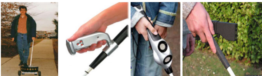
Fig. 1 From left to right Robotised smart cane, smart cane (K-Sonar), intelligent canes (UltraCane, TomPouce)
