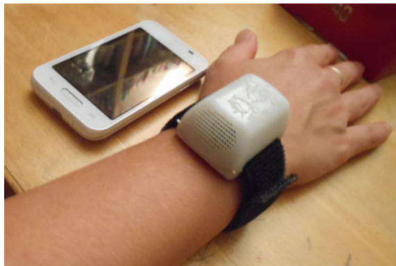
Fig. 5 ABBI bracelet together with a mobile device used to control the device settings. By default the ABBI is quiet when it is stationary, and only makes sounds when it is moved
