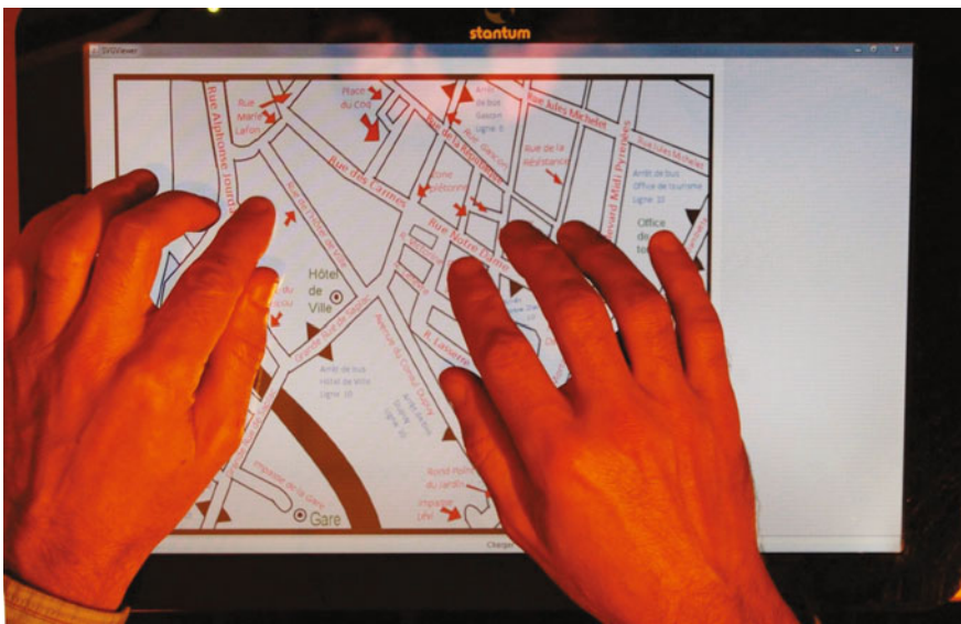
Fig. 2 Example of a Digital Interactive Map: the map content is displayed on a touch-enabled device. During exploration the device produces audio output
