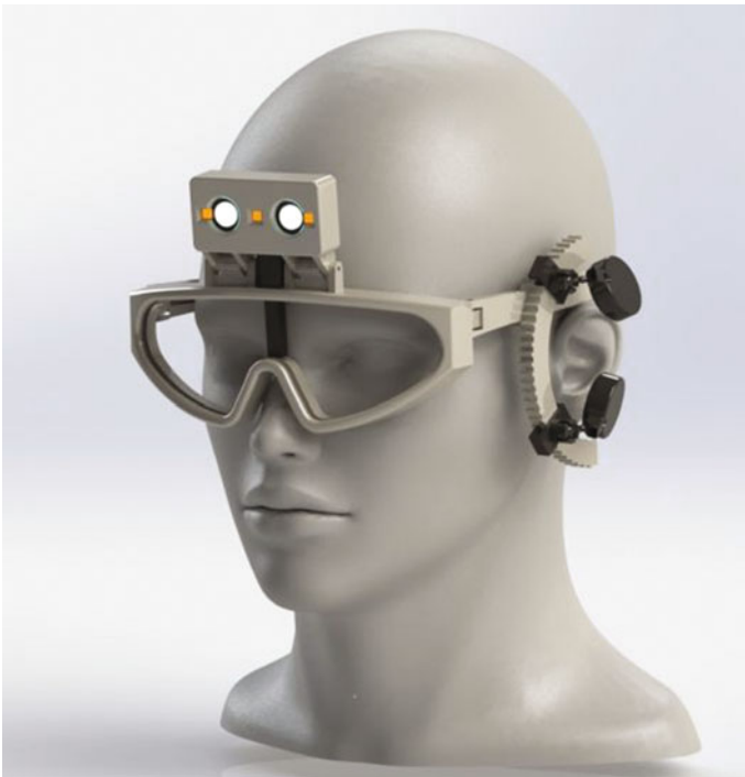
Fig. 10 Prototype proximaural quadrophonic headphones for generating spatial audio without blocking environmental sounds
