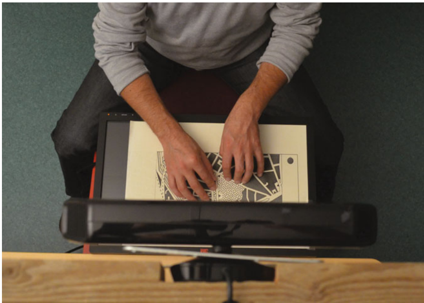
Fig. 5 Example of camera-based finger tracking combined with a raised-line map. During exploration the device produces audio output
