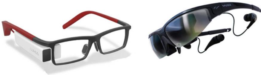
Fig. 10 Immersive and non-immersive devices. Left Lumus (Lumus Ltd) augmented reality device with see-through display screens. Right Vuzix (Vuzix Ltd) virtual reality device with opaque screens
