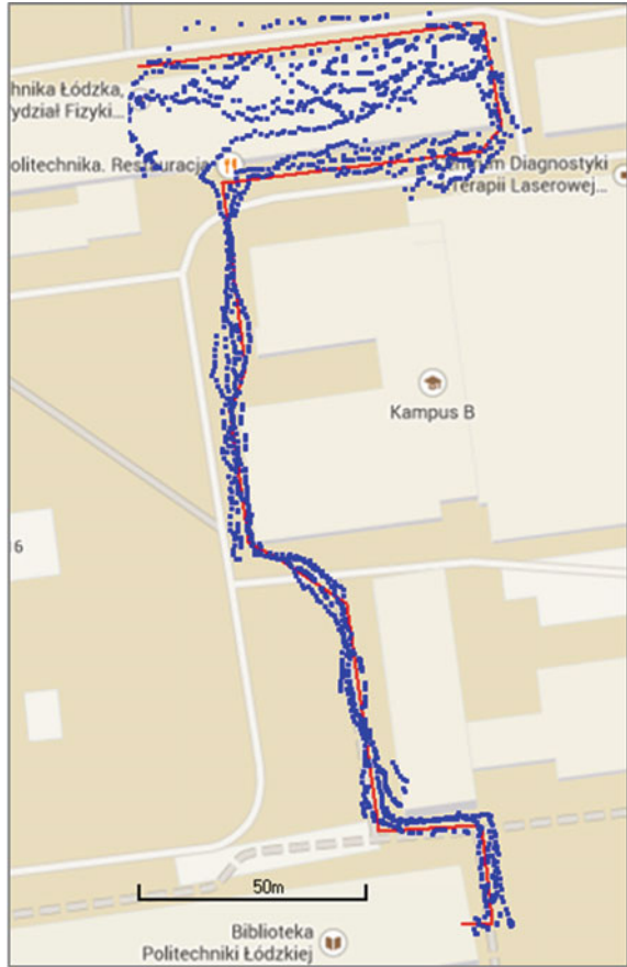
Fig. 20 An example path of 371 m length. Red solid line denotes the path followed; blue dots show GPS readouts
