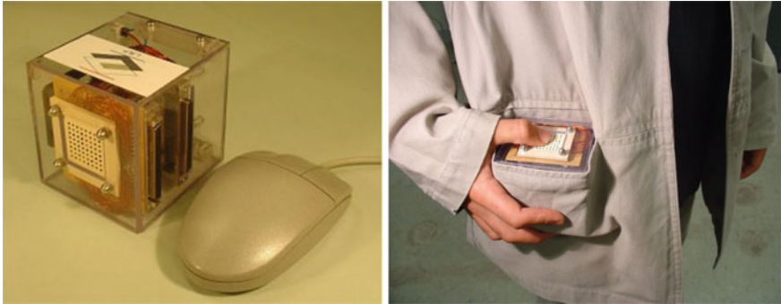
Fig. 5 TactiPad, a touch-stimulating refreshable tangible multimodal interface
