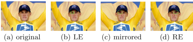
Fig. 6. (a): Input image; (b): Left eye detection; (c): Left eye detection in mirrored image; (d): Right eye detection mapped back to the original image.
