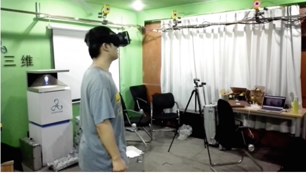
Fig. 2. The free walking VR environment using the motion capture system. The smartphone display is put in a helmet, on which four marker balls are stuck.
