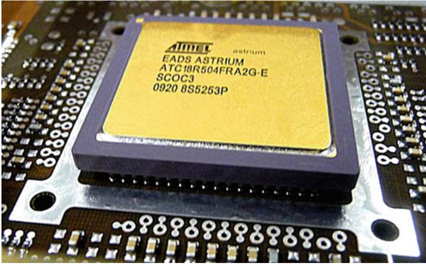
Fig. 5 SCOC3 ASIC (courtesy AIRBUS DEFENCE and SPACE)
