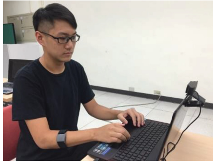
Fig. 3. The experimental environment of the first and the second studies. The camera was mounted on the computer in front of the participants. Scosche Rhythm+ is banded on participants' wrist to get the heart rate data simultaneously when being video recorded.
