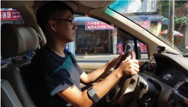
Fig. 4. The experimental environment of the third study. The camera was mounted on instrument panel below the front of the driver. Scosche Rhythm+ is also banded on participants’ wrist to get the heart rate data simultaneously when being video recorded.
