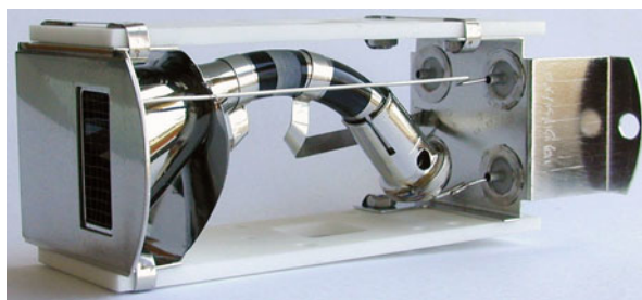
Fig. 4.95 Channeltron multiplier. Ions or electrons from a conversion dynode would enter from the left side. Amplification of secondary electrons occurs down the bent tube
