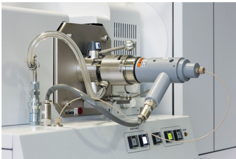
Fig. 5.9 A direct insertion probe on a JEOL AccuTOF GCx instrument. The probe is shown in its fully inserted position. The transparent hose ( left ) provides rough vacuum to the lock before insertion of the probe, the gray cable connection serves for heater power supply and temperature control, and the light brown capillary delivers pressurized gas for cooling the probe tip if required
