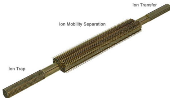
Fig. 4.90 Waters TriWave as incorporated in Synapt G2 instruments for ion mobility separation. Ions entering from the left are accumulated in the first section acting as the ion trap, then batch wise admitted into the ion mobility separation zone, and finally collected for transfer into the oaTOF analyzer (Adapted with permission. Courtesy of Waters MS Technologies)
