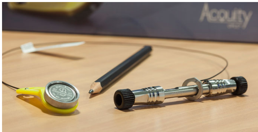
Fig. 14.8 UPLC column. The actual column ( right ), here shown with the two end caps still in place, is quite small as by comparison to the pencil. This particular column is a Waters BEH C18 reversed phase type of 50 mm length and 2.1 mm inner diameter filled with 1.7- \mu\text{m} -sized particles. The column is locked to a transponder ( left ) that is used to identify the column by the data system
