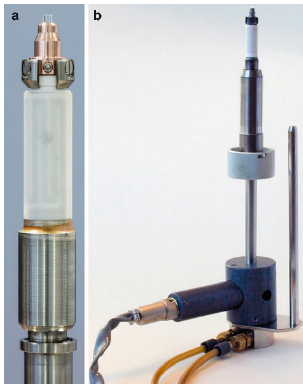
Fig. 5.7 Direct insertion probe (DIP) for use with EI, chemical ionization (CI), and field ionization (FI). (a) The copper probe tip holds the glass sample vial and is fitted to a temperature-controlled heater. The heater, a thermocouple, and cooling are provided inside. The (white) ceramics insulator protects the operator from the high voltage of the ion source. (b) Entire DIP of a JEOL JMS-700 equipped with water cooling
