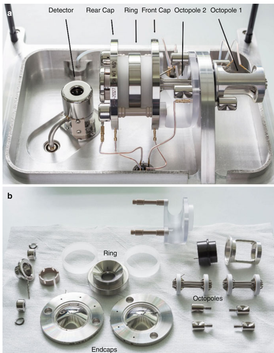
Fig. 4.62 Analyzer maintenance of a QIT; here of the Finnigan LCQ. (a) Complete QIT analyzer mounted onto the top cover plate of the vacuum manifold, (b) after taking it apart for cleaning
