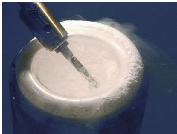
Fig. 10.18 Getting ready for LT-FAB by immersion of a FAB target with sample solution into liquid nitrogen. After about 30 s the solvent matrix is deeply frozen and the tip is cooled to allow for transfer of the probe into the vacuum lock and further into the ion source whilst avoiding untimely thawing of the solvent
