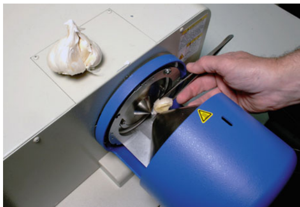
Fig. 13.31 Commercial DART source of the first generation on a JEOL AccuTOF instrument. Here it is used for the analysis of volatiles from a garlic clove [125, 126]. The sample is simply held into the open gap between the metastable atom source ( lower right part ) and the orifice of the API interface ( upper left ). Photograph by courtesy of JEOL USA
