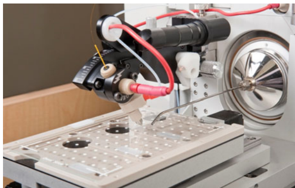
Fig. 13.3 A commercial DESI ion source. This one here is the Prosolia Omni Spray 2D source coupled to a Thermo Fisher LTQ mass spectrometer. The surface shown is a 96-spot Omni Slide HC having the standard microtiter plate dimensions. Note the extended desolvation capillary and the adjustable sprayer (Courtesy Prosolia, Inc., Indianapolis, IN USA)
