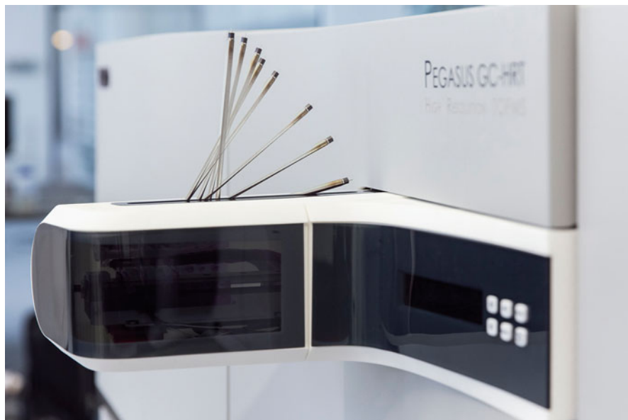
Fig. 5.13 Automated DIP in operation as visualized by multiple exposures. After having received the sample vial in vertical orientation, the rod is driven to the left and tilted downward for insertion through the lock. The photograph shows the SIM DIP mounted to a LECO Pegasus GC-HRT instrument
