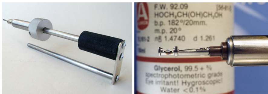
Fig. 10.6 FAB probe of a JEOL JMS-700 magnetic sector instrument ( left ). The probe tip with a drop of glycerol placed onto the exchangeable stainless steel FAB target ( right )
