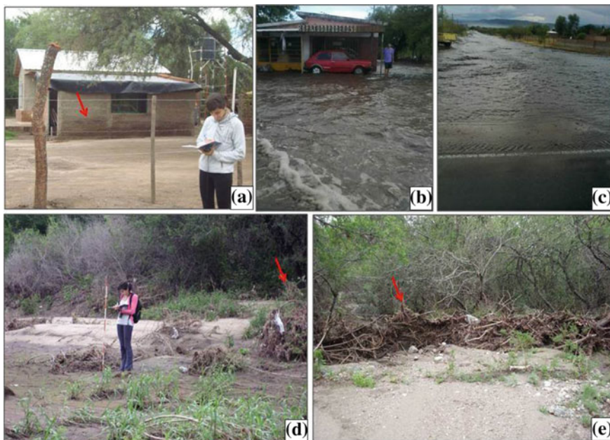
Fig. 10 Water height during the flash flood (a, b, c) and water-level marks considering the vegetation (d, e). Photograph locations in Fig. 9: a P4, b and c P5, d P1, e P3
