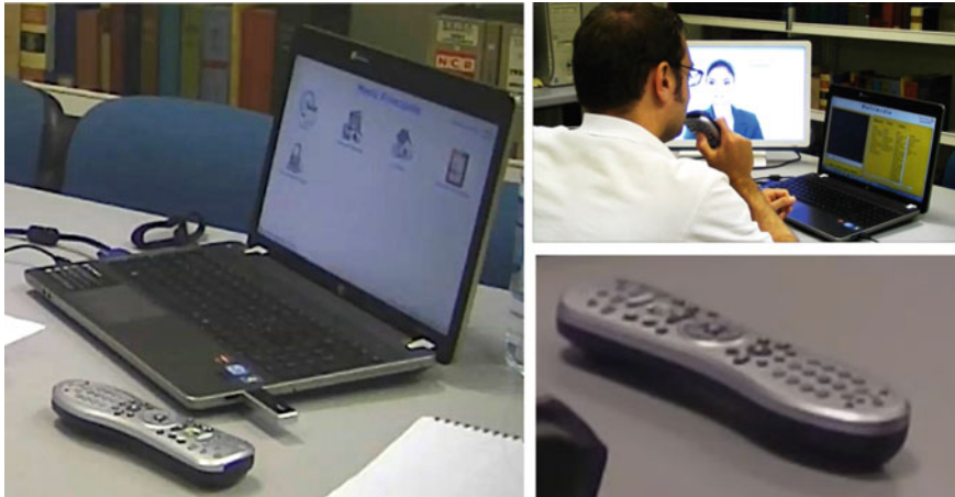
Fig. 4 The SPEAKYACUTATTILE devices. On the left , the remote controller connected to the pc via USB is displayed, while on the right it is possible to see the Speaky Avatar
