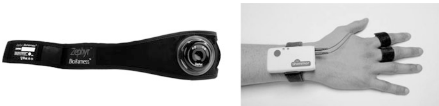
Fig. 1 Zephyr BioHarness™3 on the left and Shimmer GSR Sensor on the right
