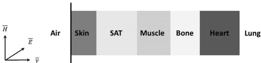
Fig. 1 The multilayer EM model proposed to study the interaction between an EM wave and human chest
