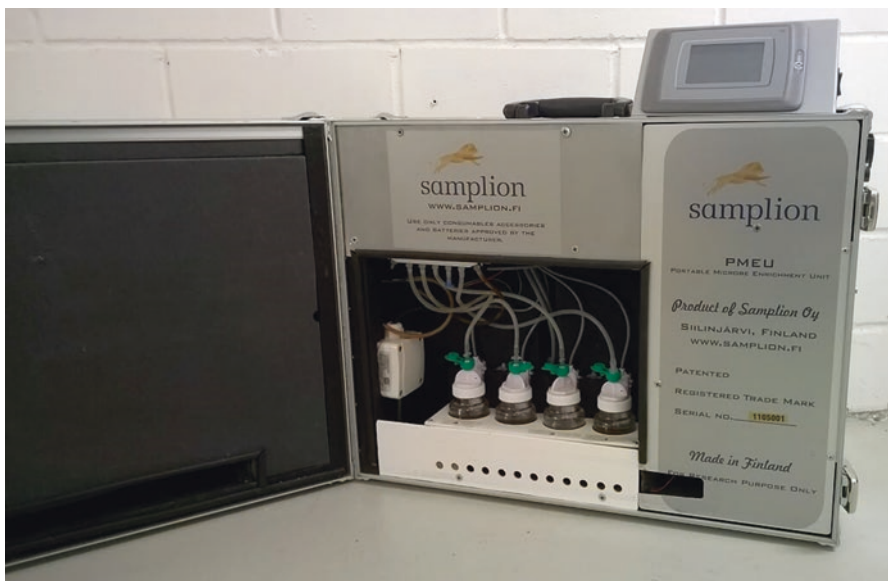
Fig. 7.5 PMEU Coliline™ unit is equipped with Automated Sample Collection System for online monitoring of clean water in water departments and in the distribution system. The unit can be connected directly to the water tubing (See also McCoy 2015). (Photograph by Jouni Pesola)
