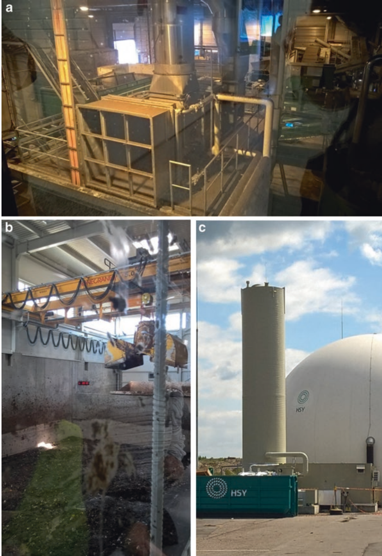
Fig. 7.4 (a) The sorted biowaste reception unit automatically handles baskets or containers from all over the cities in the Metropolitan Helsinki area with the daily waste input of around 200–250 tons. (b) Different organic wastes are homogenized and pretreated for a biogas unit. (c) Biogas is one of the main products of the HSY waste treatment plant in Ämmässuo, Espoo, close to the border with Helsinki. (Photographs by Elias Hakalehto)
