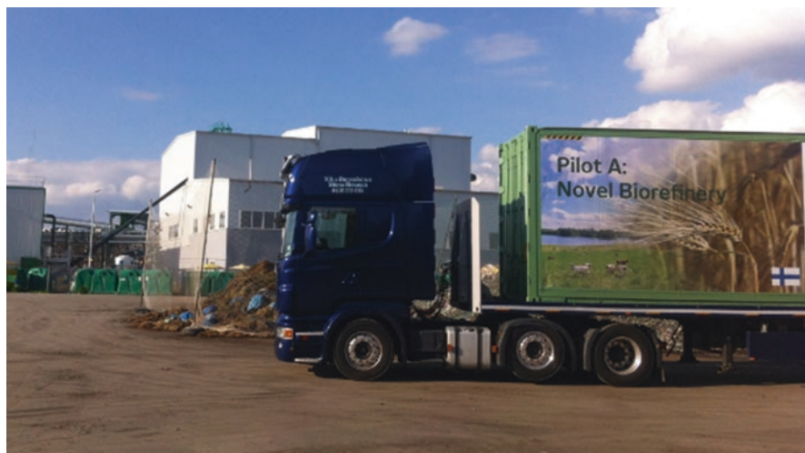
Fig. 7.6 Pilot A Novel Biorefinery arriving at its Polish testing site at ZGO Gać Ltd's waste management centre in Lower Silesia. Industrial levels of microbial metabolites, such as organic acids, alcohols and hydrogen, were obtained from the carboxylate wastes of food industries, as well as sorted biowaste. For a survey of the results, see den Boer et al. (2016a, b; Hakalehto et al. 2017a) or www.abowe.eu (Photograph by Mika Ruotsalainen)
