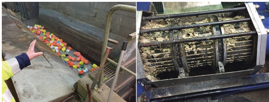
Fig. 4.35 Household waste sorted into different coloured bags and sorted automatically in Eskilstuna. The organic household waste is pressed through the press to the right, and the material that passed is used as feed stock to the fly larvae production (Photo Erik Dahlquist)
