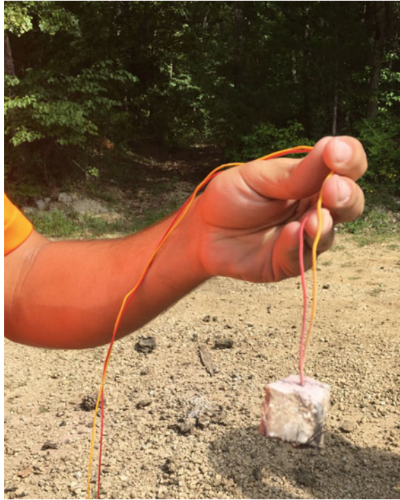
Fig. 3.6 Stemming plug formation with free flowing solids
