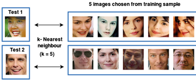
Fig. 2. k -nearest neighbours computed for two unlabelled test samples: Michelle Wie and Ben Stiller. From the training set of 5 seen classes, k -nearest neighbour ( k = 5 ) based on the Euclidean distance from the test image is seen. The neighbors selected depends on attributes. Attributes like the shape of face and age is similar for the nearest neighbors in this example.
