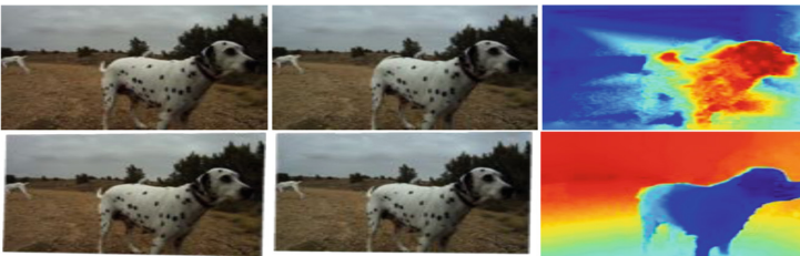
Fig. 3. Sample disparity estimation. The first two columns are the original stereo pair and their rectified images. The top-right picture is the disparity map computed by [36], the bottom-right is the depth map obtained by optical flow [37] between the left and right view.
