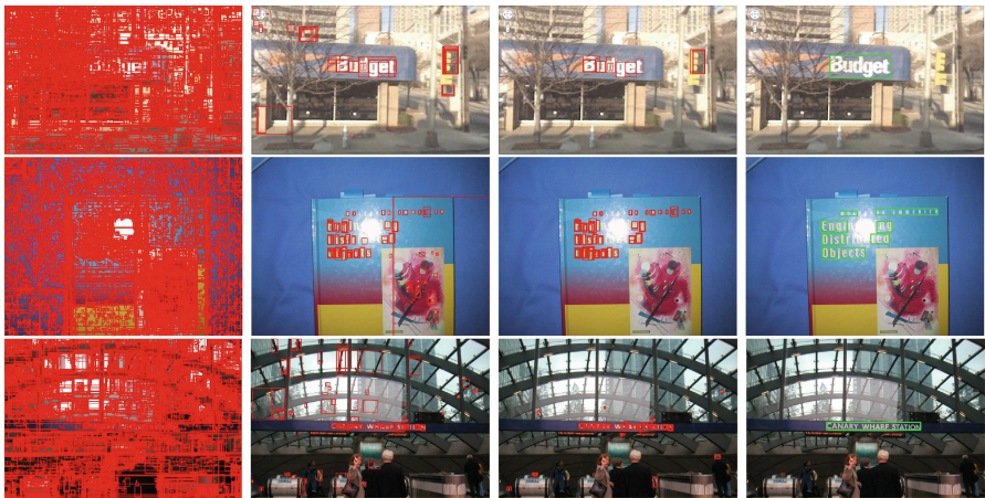
Fig. 2. Images from the scene text detection pipeline. From left to right: (1) Region proposals; (2) Coarse predictions; (3) Predictions after aggregating local context; (4) Final detected text lines.
