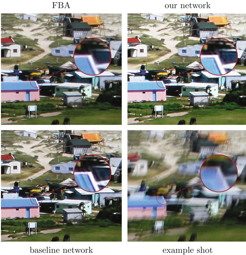
Fig. 9. Comparison to a baseline approach of simply stacking [3,11]. Without end-to-end training ringing-artifacts are clearly visible on the blue roof. They are significantly dampened after training. (Color figure online)
