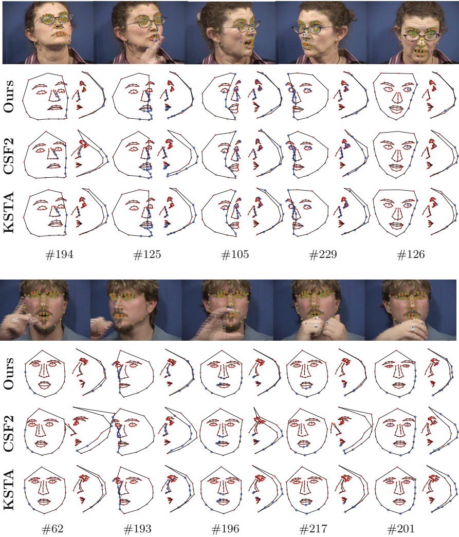
Fig. 5. ASL database. In each row we show the same information. Top: 2D tracking data and reconstructed 3D shape reprojected into several images with green circles and red squares, respectively. Blue squares correspond to missing points. Bottom: Camera frame and side-views of the reconstructed 3D shape: our solution, CSF2 [20] and KSTA [6], respectively. We also represent the number of image k in the input data, showing as different objects are intercalated. Best viewed in color.
