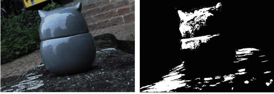
Fig. 2. The left image shows the center view of a light field captured with a Lytro Illum camera. The right image shows the specular mask obtained by our method.
