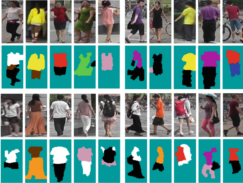
Fig. 2. Some examples of labeled images in the Pedestrian Color Naming dataset. The images in the first row are the original images and those in the second row are the color label maps where each region is visualized using the corresponding basic colors (black, blue, brown, grey, green, orange, pink, purple, red, white, and yellow). The background region is shown in dark cyan. (Color figure online)
