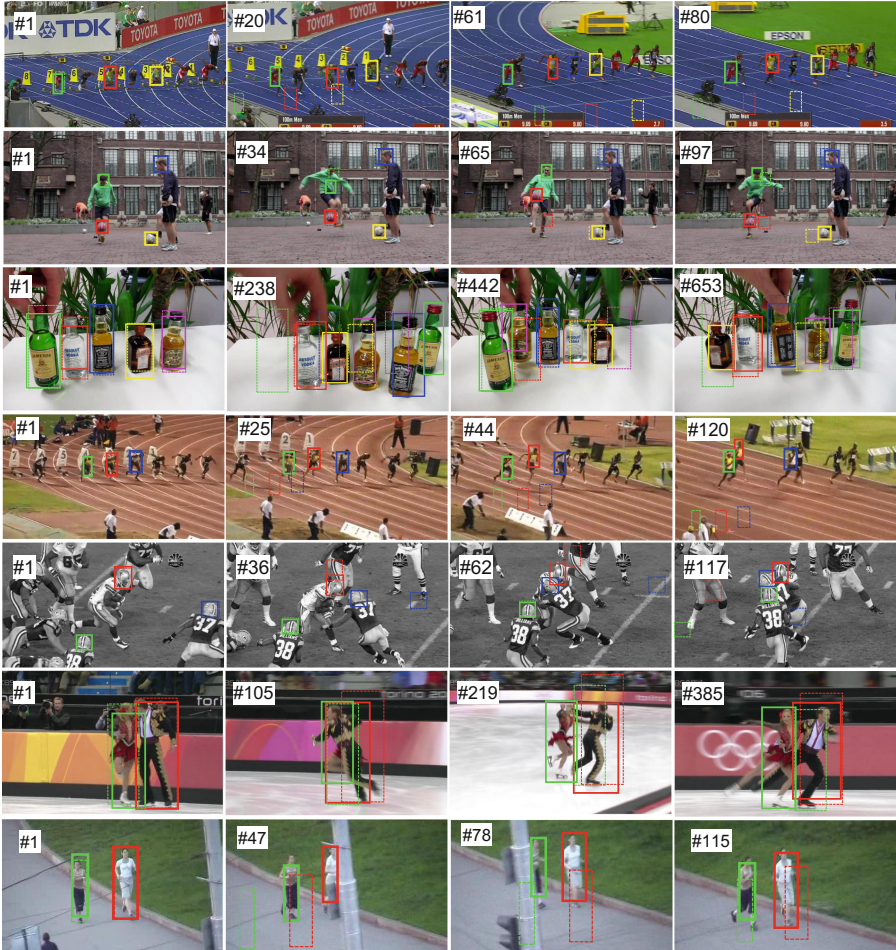
Fig. 5. Qualitative comparisons with the proposed PMOT tracker (solid lines) against the SPOT tracker (dash lines) on videos “bolt1”, “ball1”, “liquor”, “bolt2”, “football”, “skating2” and “jogging” from MOOT dataset (from top to bottom). Our method exhibits robustness in challenging scenarios such as repetitive mutual occlusions and similar target appearances.
