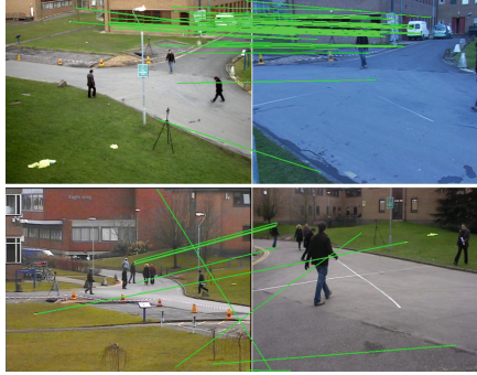
Fig. 4. Top: Only frame pair of PETS2009 with an inlier-only correspondence set. Bottom: Typical failure containing overfitted outliers.eps
