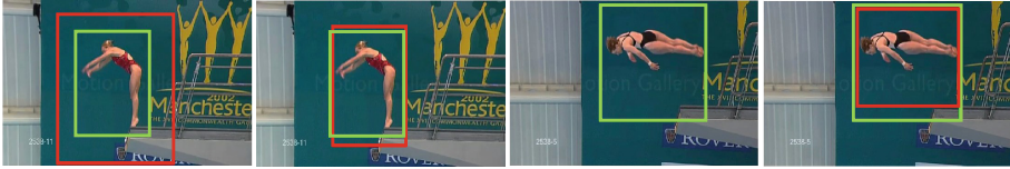
Fig. 2. Comparison of human detection results. The bounding boxes with red and green color are the ground truth and the detection results respectively. The 1-st and 3-nd columns are from the initial Faster R-CNN [18] (There is a missing detection in the 3-nd column); while the 2-nd and 4-th columns are from our fine-tuned model. (Color figure online)
