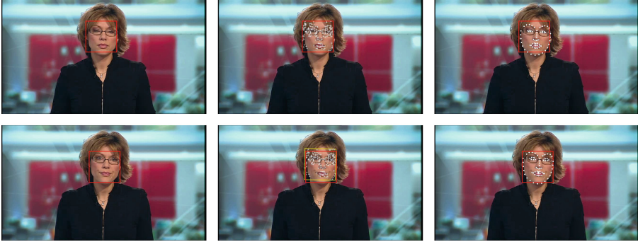
Fig. 4. Left: face detections; Middle: KLT features and the tracked bounding box (in yellow); Right: facial landmarks. (Color figure online)
