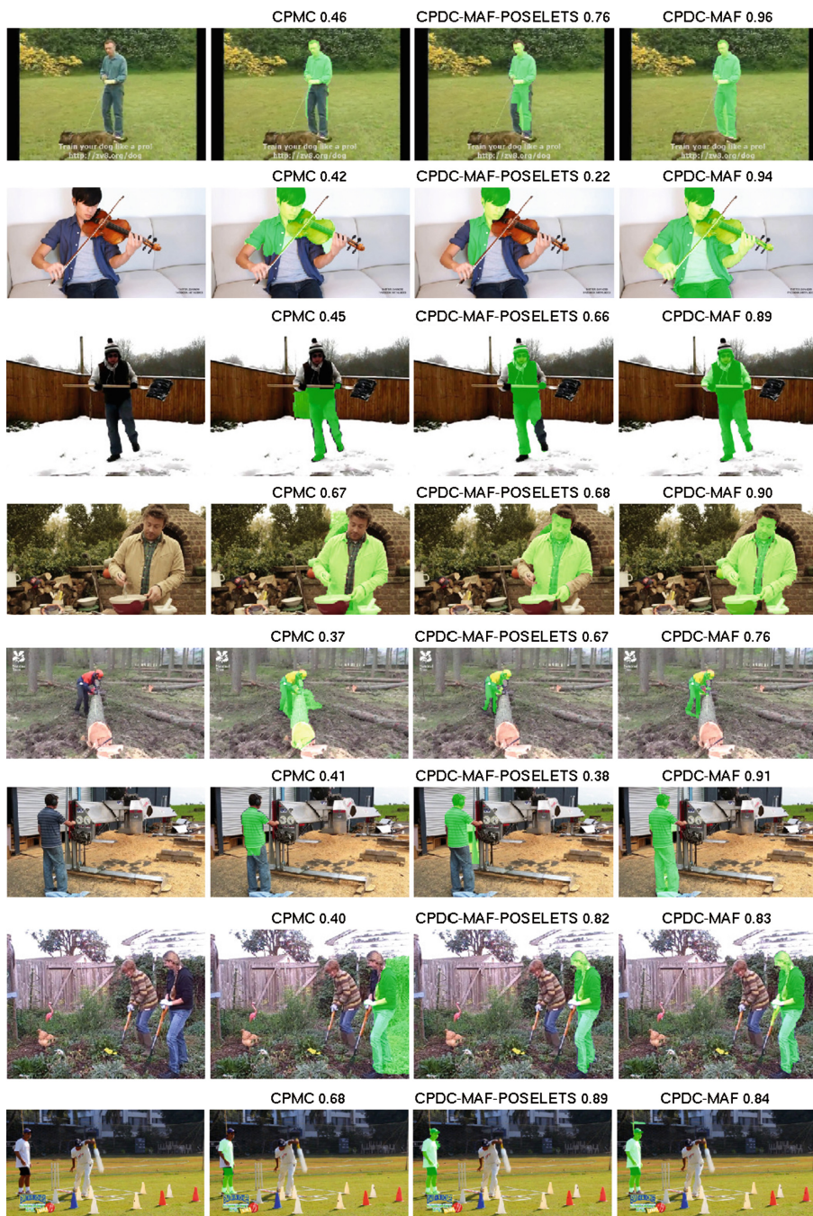
Fig. 6. Segmentation examples for various methods. From left to right, original image, CPMC with default settings on person's bounding box, CPDC-MAF-POSELETS and CPDC-MAF. See also Table 1 for quantitative results.
