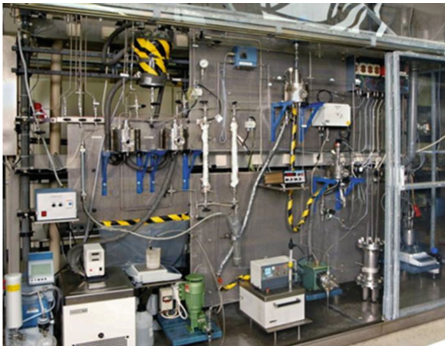
Fig. 8.6 Picture of the continuously operated miniplant for the telomerisation of butadiene with glycerol
