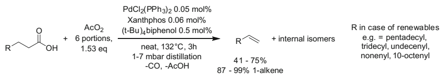
Fig. 7.38 Grubbs' protocol for decarbonylative dehydrogenation of saturated fatty acids
