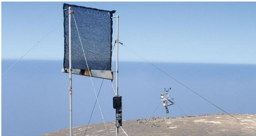
**Fig. 14.2** SFC—Standard Fog Collector, Alto Patache, Atacama (photo: *Martino Correggiari, 2012*)
