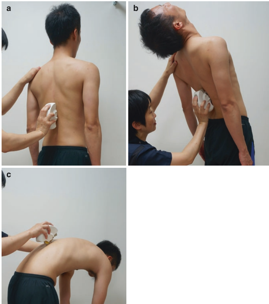
Fig. 3.3 SpinalMouse®. Not only the curvature of the spine (a) but also the mobility of the spine (b, c) can be measured with this device. Our original photos
