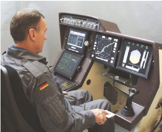
Fig. 9.121 Experimental cockpit with touch pad installed at the right armrest
