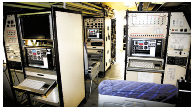
Fig. 9.53 ATTAS upgrade—flight data display on all work stations
