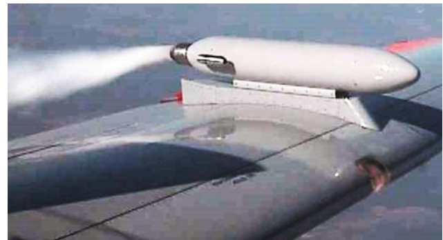
Fig. 9.111 Smoke generator on ATTAS left wing
