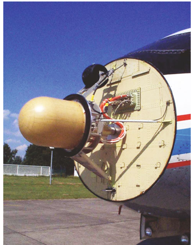
Fig. 9.87 Millimeter wave radar and infrared sensor on ATTAS
