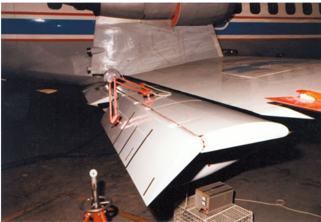
Fig. 9.31 Calibration of DLC flap deflection
