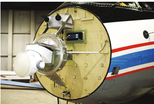
Fig. 9.98 Sense and avoid sensor integration in ATTAS
