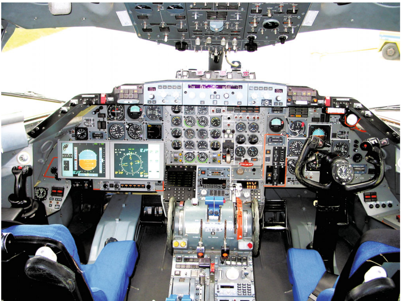
Fig. 9.47 ATTAS upgrade—flat screens in cockpit
