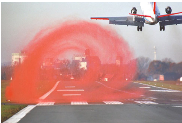
Fig. 9.110 Visualization of ATTAS wake flow field
