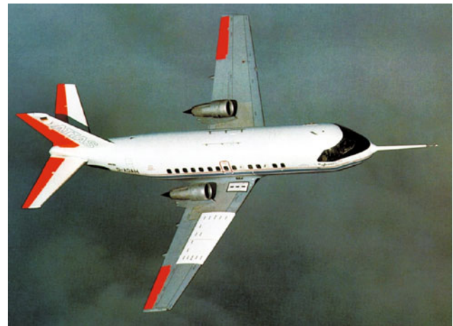
Fig. 9.11 Aerodynamic investigation with laminar flow glove
