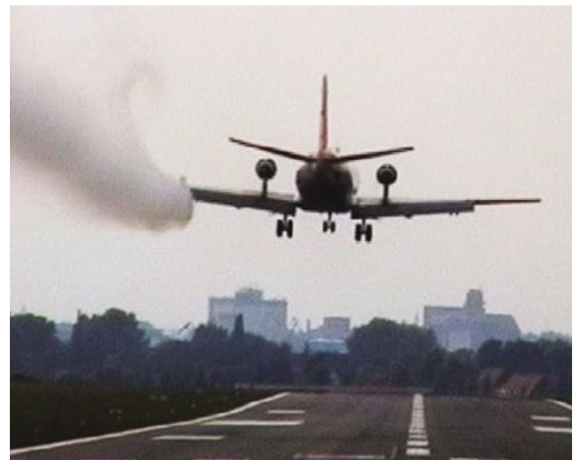
Fig. 9.112 Visualization of left wake vortex of ATTAS
