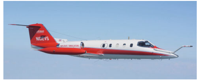
Fig. 5.30 Calspan Gates Learjet model 25B N102VS with a refueling nose probe
