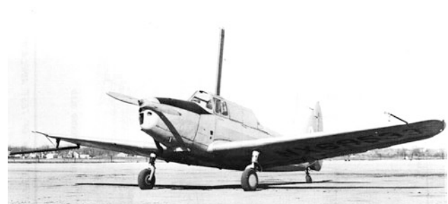
Fig. 5.4 Fairchild PT-26 with vertical boom
