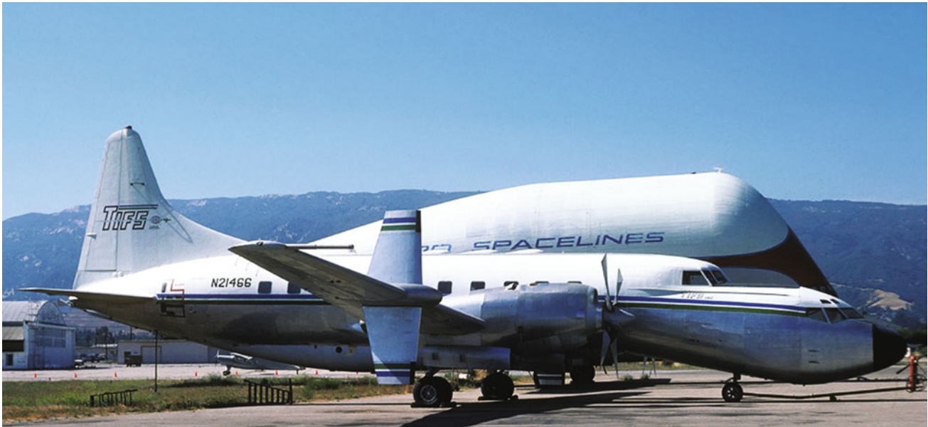
Fig. 5.20 Convair 580 TIFS II with civilian registration number and Boeing 707 nose (Credit Peter de Groot)
