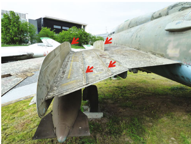
Fig. 4.5 Sukhoi Su-22UM3 K—oversized boundary layer fences
