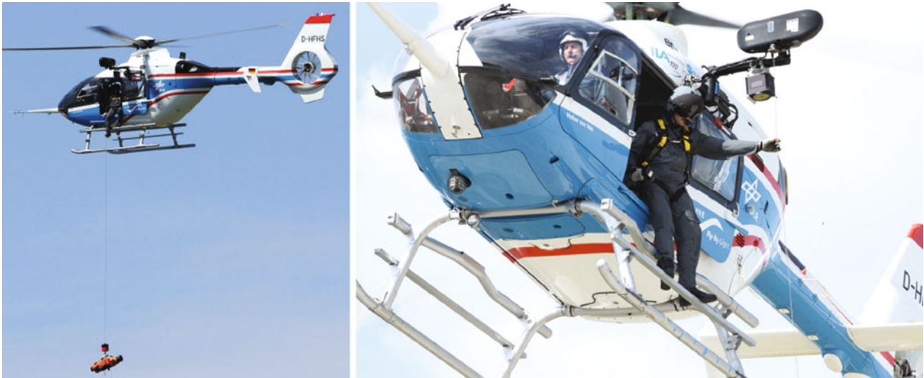
Fig. 10.38 Flight test for sling load assistance system with load motion sensor
