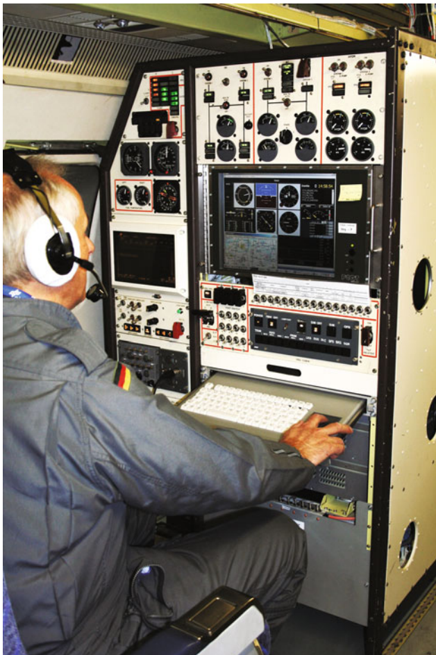
Fig. 9.52 ATTAS upgrade—flight test engineer Michael Preß on FI cabinet with new operating console and display
