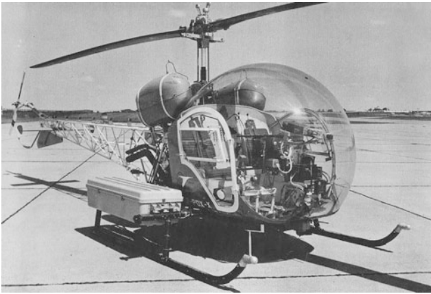
Fig. 5.73 NRC Bell 47G3B-1 airborne simulator
