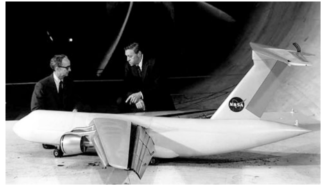
Fig. 6.105 John P. Campbell, left, inventor of the externally blown flap (EBF) concept, and Gerald G. Kayten, of NASA Headquarters, pose with a generic free-flight model of an STOL configuration at the Langley full-scale wind tunnel (Credit NASA)
