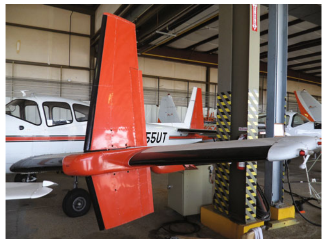
Fig. 5.70 UTSI Navion (R/N N55UT) with side force generators
