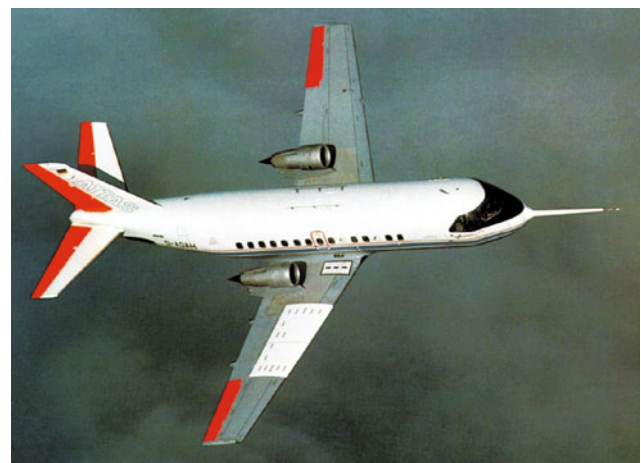
Fig. 9.11 Aerodynamic investigation with laminar flow glove
