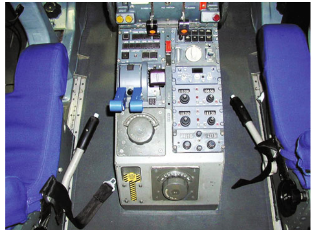
Fig. 9.17 Center console with VBG, experimental thrust and flap levers
