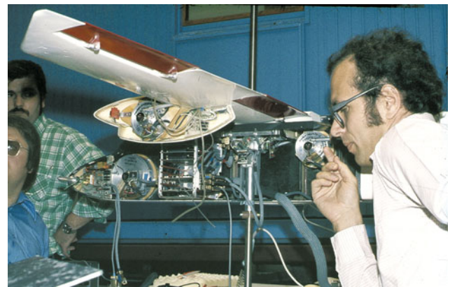
Fig. 6.112 Actuators and signal processing onboard the wind tunnel model (1976, on the right Rüdiger Karmann)
