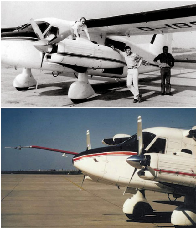
Fig. 6.93 Do 28D Skyservant with nose boom and flight log
