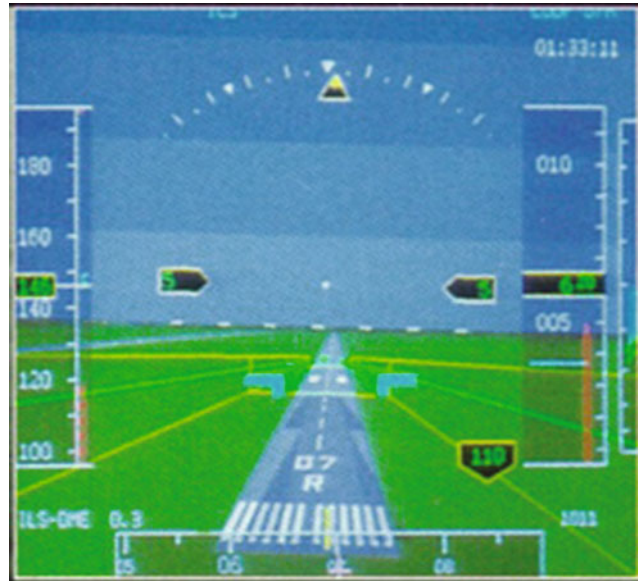
Fig. 9.79 Display in PFD: during final landing
