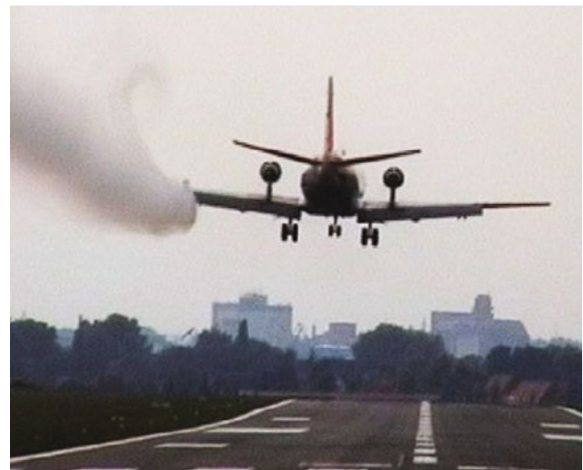
Fig. 9.112 Visualization of left wake vortex of ATTAS
