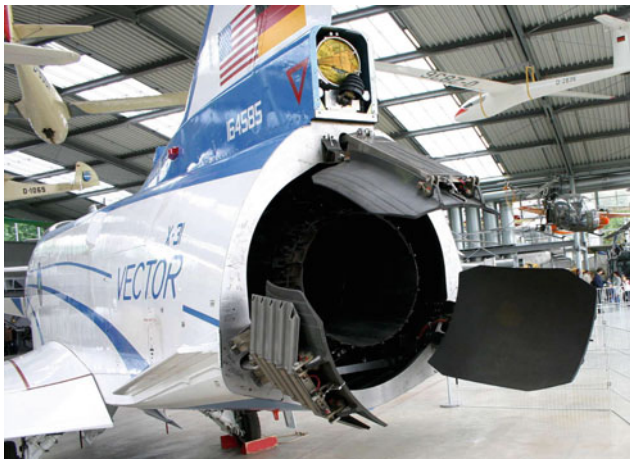
Fig. 6.150 Boeing-EADS X-31 VECTOR graphite composite thrust vector deflectors (Credit www.456fis.org )
