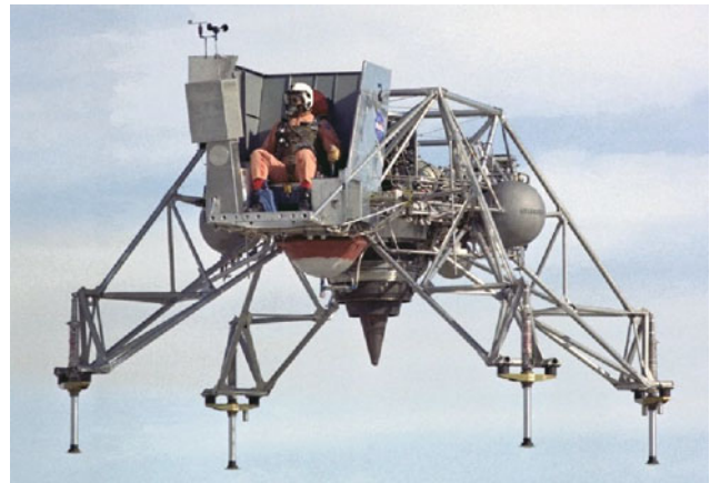
Fig. 6.10 NASA Lunar Landing Research Vehicle (LLRV) with cockpit casing
