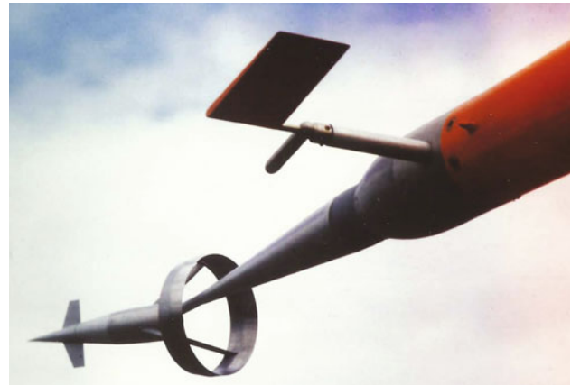
Fig. 7.23 Flight log with angle of attack vane
