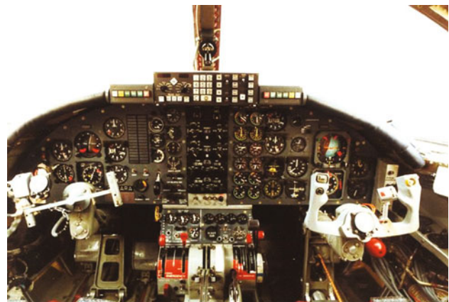
Fig. 7.45 IFGS experimental cockpit equipment
