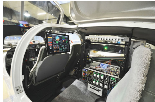
Fig. 6.159 Rear cabin view of FTE workstation and flight control system electronics
