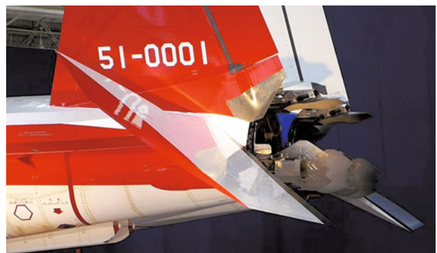
Fig. 6.76 ATD-X twin engine thrust vector paddles (Credit AFP screencap)
