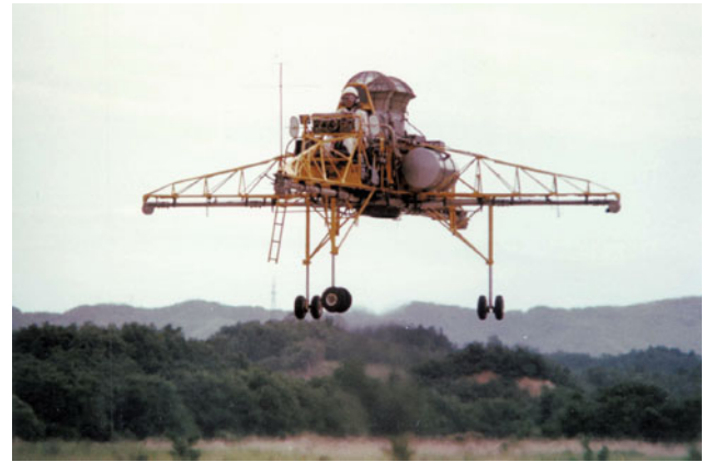
Fig. 6.15 NAL VTOL flying test bed (front view)
