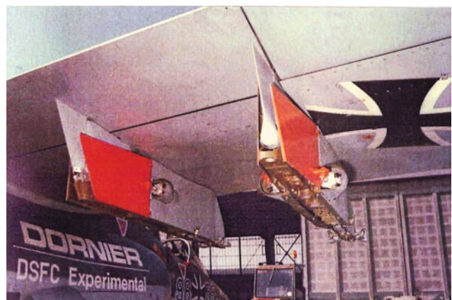
Fig. 6.126 Electrohydraulically driven pylon split flaps
