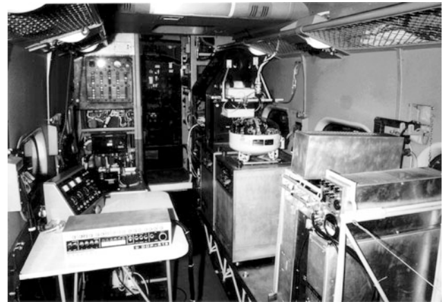
Fig. 6.88 Components of digital FBW control in the Pembroke cabin ( right , from front: digital computer, two hydraulic systems, inertial platform LN3, left , input console for digital computer, central operating desk for hydraulic system, triplex actuator drive)
