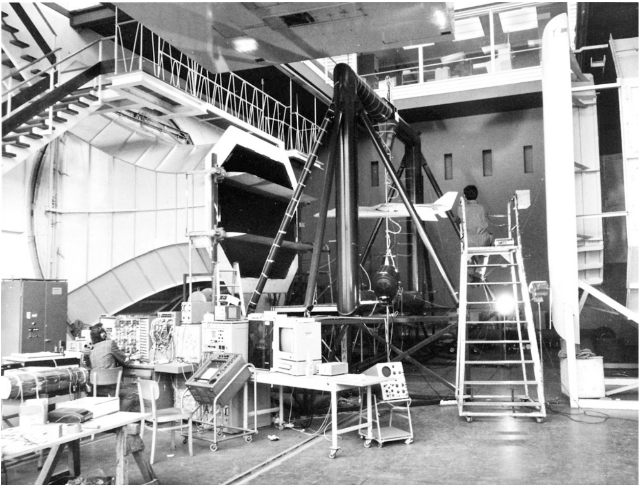
Fig. 6.106 Facility for dynamic simulation in wind tunnel with BASE-Model
