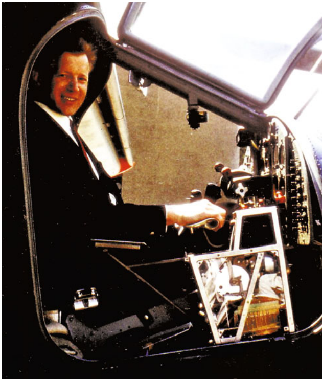
Fig. 6.86 Control inputs in Do 27 through a sidegrip inceptor by Johannes Tersteegen
