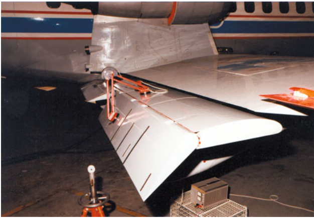
Fig. 9.31 Calibration of DLC flap deflection
