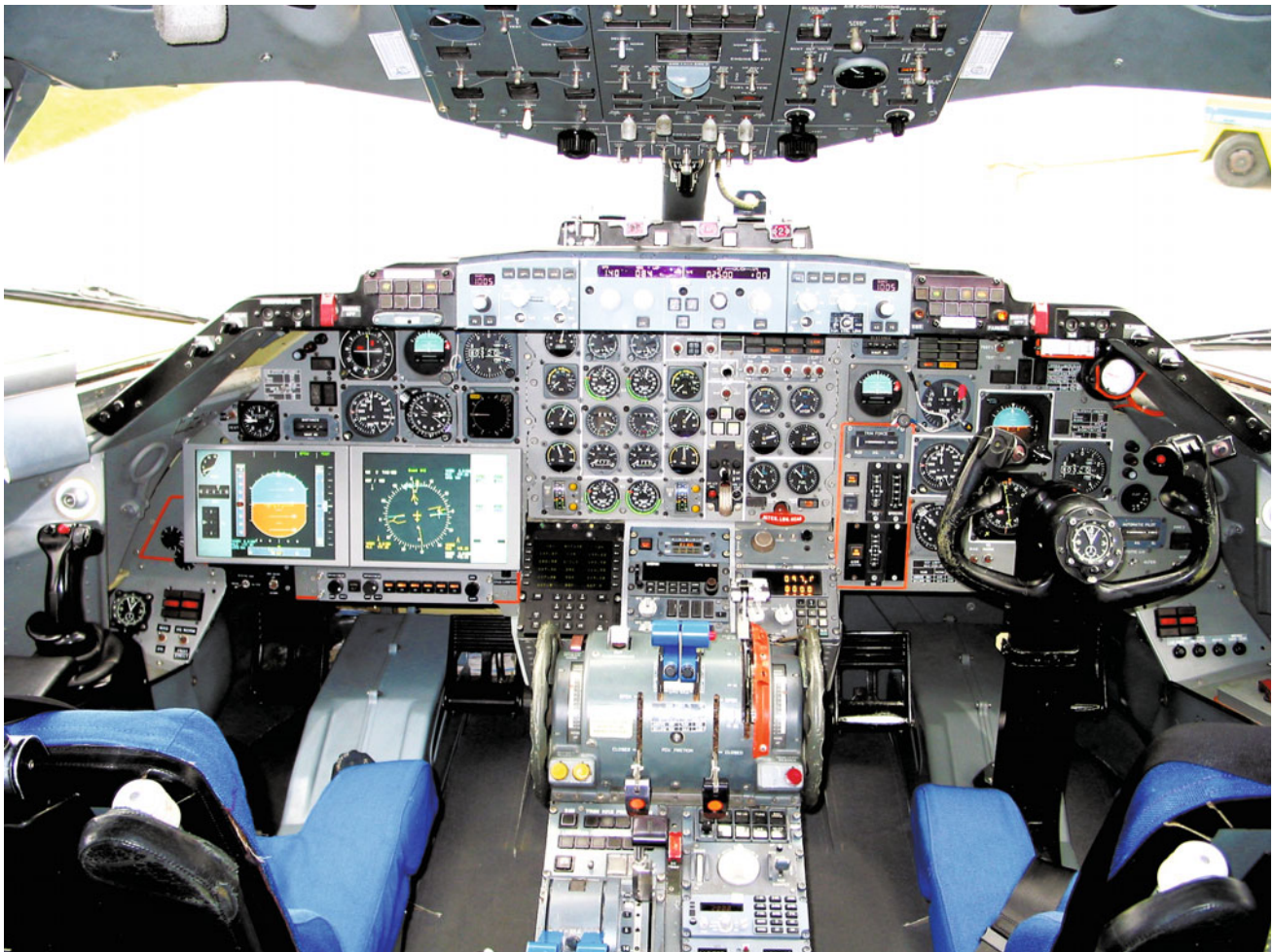
Fig. 9.47 ATTAS upgrade—flat screens in cockpit
