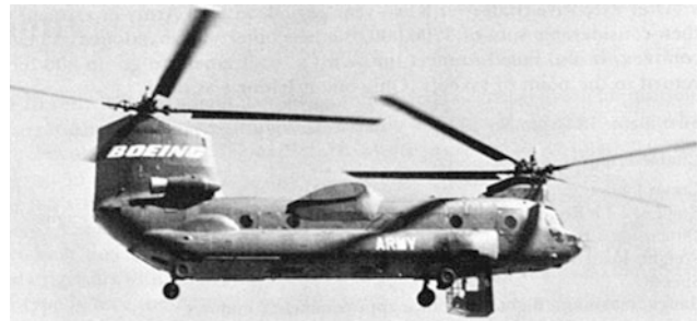
Fig. 6.31 Boeing-Vertol BV 347 as HLH-Fly-by-Wire demonstrator
