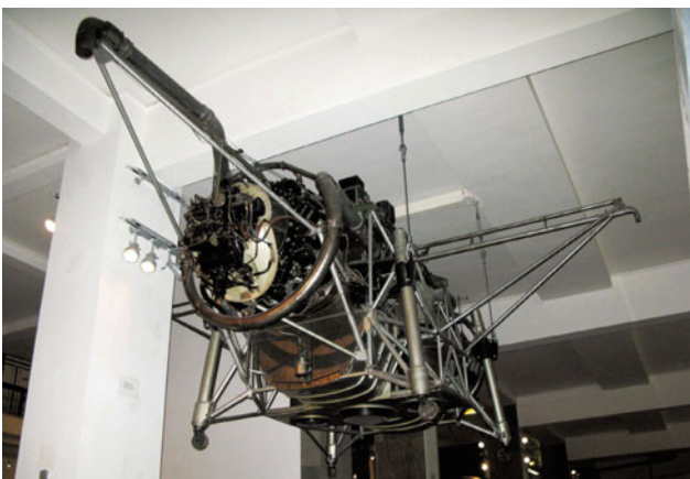
Fig. 6.9 Rolls-Royce thrust measuring rig TMR in Science Museum, London
