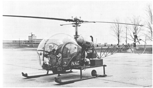
Fig. 5.72 NRC Bell H-13G airborne simulator
