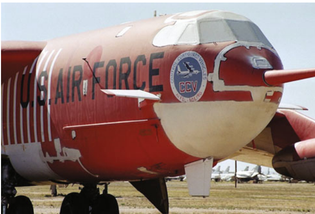
Fig. 6.33 Boeing NB-52E CCV with canard control surfaces on fuselage
