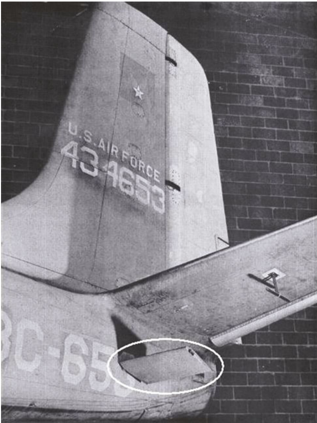
Fig. 5.7 JTB-26B auxiliary rudder surfaces
