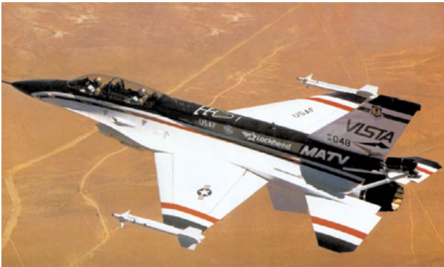
Fig. 6.48 General NF-16D MATV with anti-spin devices on tail
