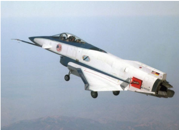
Fig. 6.134 X-31A quasi-tailless with extended airbrakes
