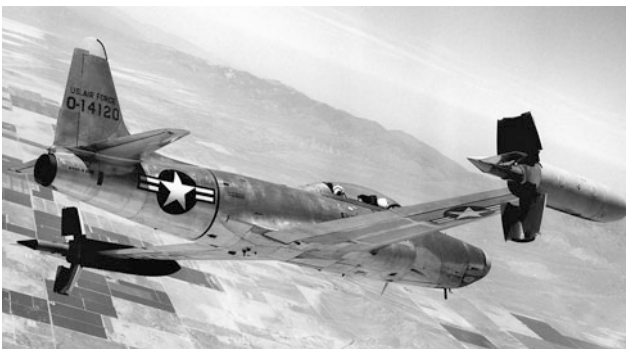
Fig. 5.12 NT-33A during X-15 steep approach simulation
