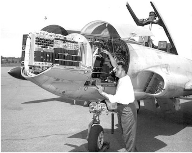
Fig. 5.11 NT-33A with EF-94A nose
