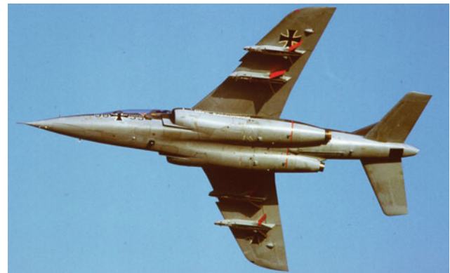
Fig. 6.128 DSFC test aircraft with deflected pylon split flaps
