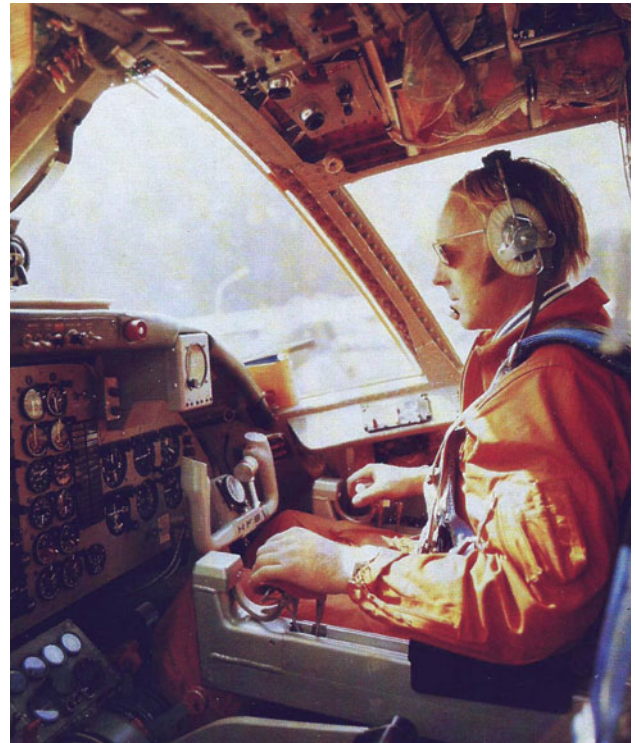
Fig. 7.17 Sidegrip operating unit for pitch and roll control (“HaLu” Meyer in cockpit)
