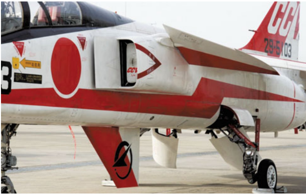
Fig. 6.73 Mitsubishi T-2 CCV with additional control surfaces
