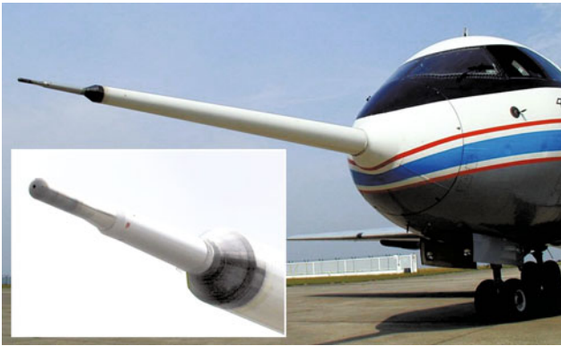
Fig. 9.48 ATTAS upgrade—5-hole probe for air data
