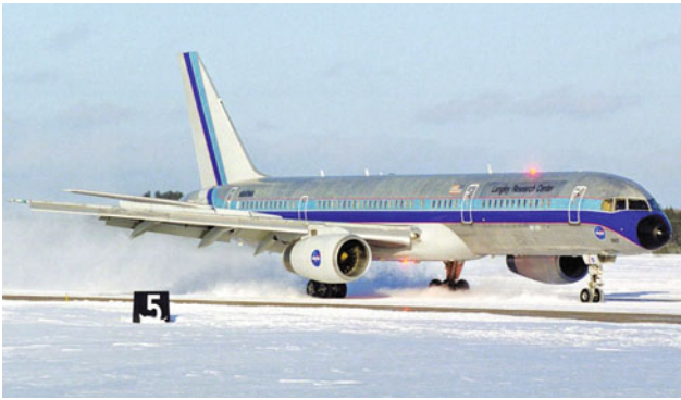
Fig. 6.47 Boeing B 757 ARIES during taxi test on snow
