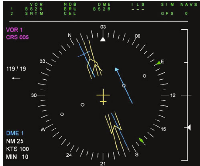
Fig. 9.123 Navigation display (Rose mode configured for VOR-navigation)
