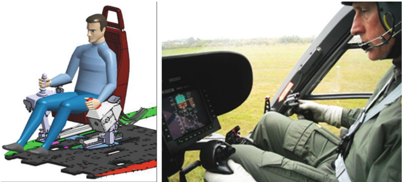
Fig. 10.29 FHS-cockpit with 2 sidesticks, side-by-side configuration
