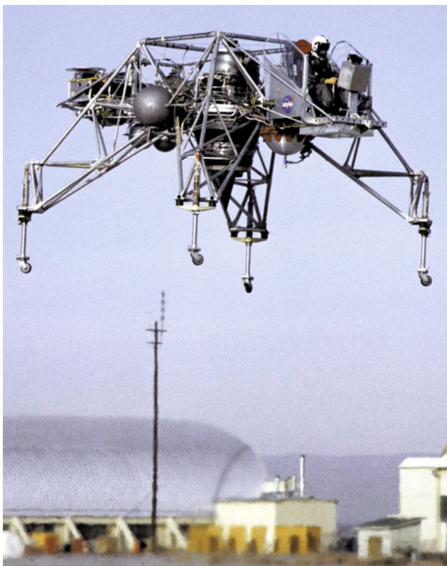
Fig. 6.11 NASA Lunar Landing Training Vehicle (LLTV) without cockpit casing
