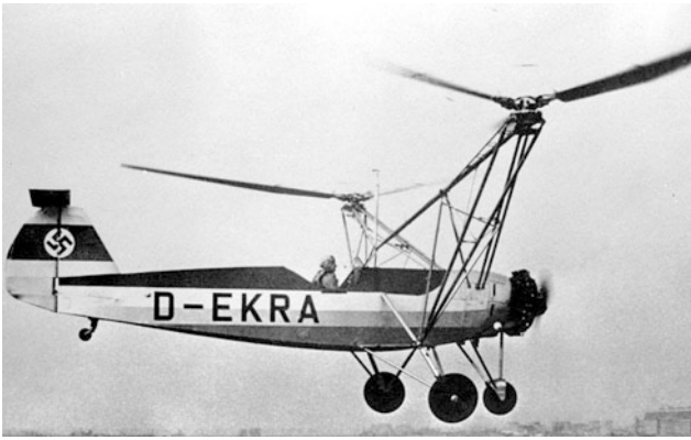
Fig. 2.10 The first ready for use helicopter Focke-Wulf Fw 61 (1936)
