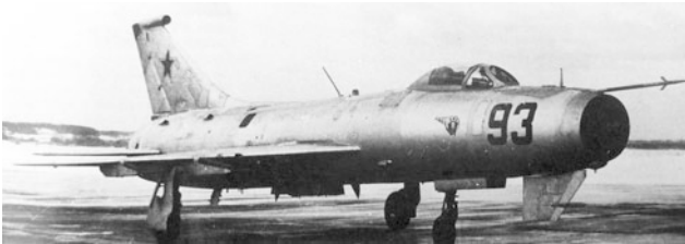
Fig. 6.61 Sukhoi L02-10 with one additional vertical control surface
