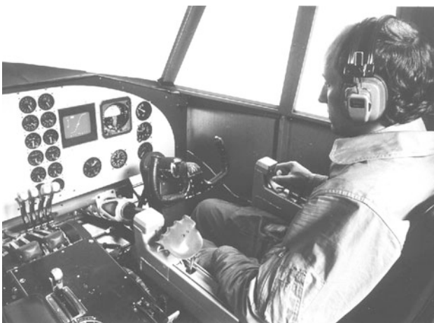
Fig. 7.43 Ground-based simulator investigations of different command control concepts for steep approaches (Volkmar Adam in cockpit)
