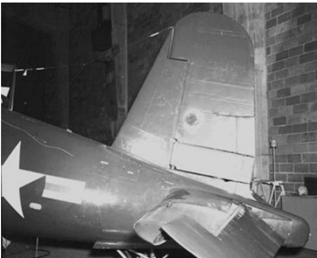
Fig. 5.3 F4U-5 split rudder
