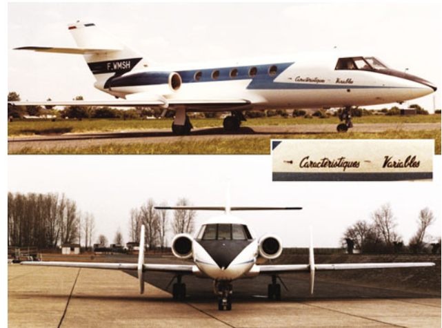
Fig. 5.81 Mystere-Falcon 20 CV without and with side force control surfaces (Credit Jean Francois Georges)
