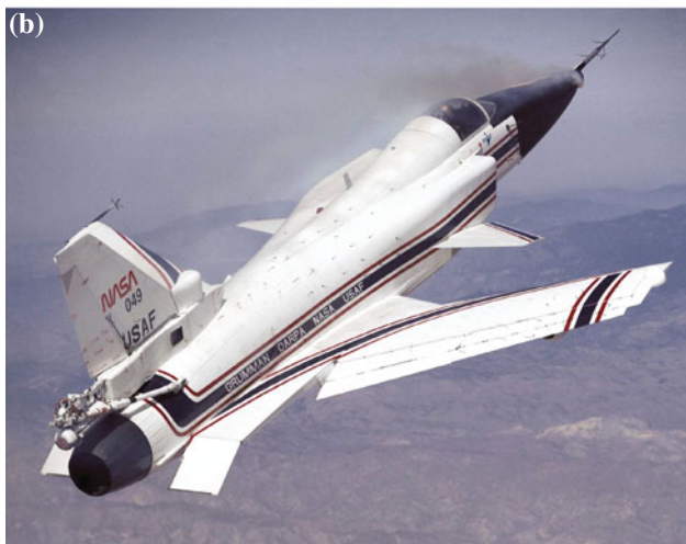
Second prototype with anti-spin devices.
