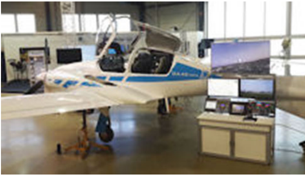
Fig. 6.160 Aircraft-in-the-Loop simulation with Ground Control Station
