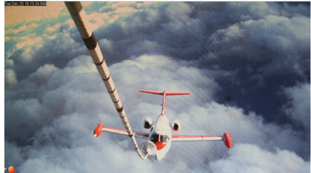
Fig. 5.31 Calspan Gates model 25B N102VS during autonomous air refueling
