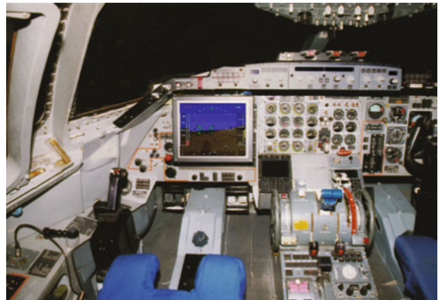
Fig. 9.80 LCD display in ATTAS cockpit for synthetic vision
