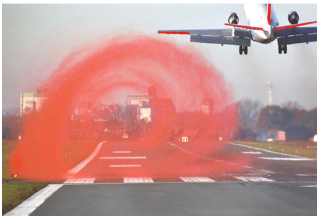
Fig. 9.110 Visualization of ATTAS wake flow field
