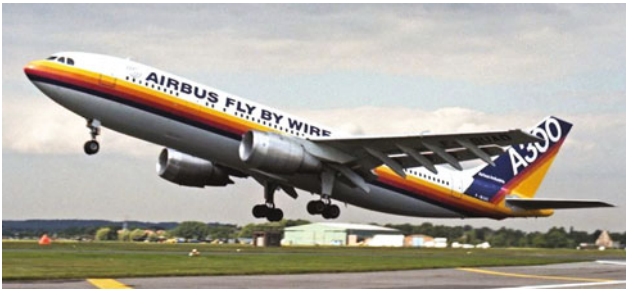
Fig. 6.70 Airbus A300 Fly-by-Wire technology demonstrator
