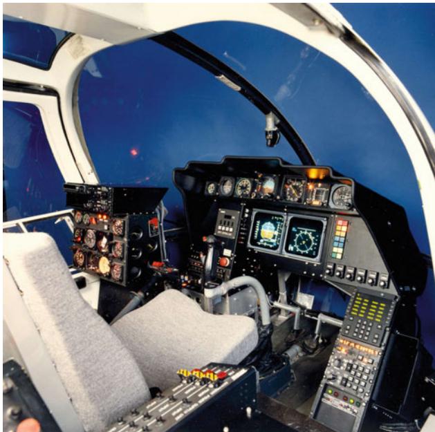
Fig. 8.28 ATTheS Cockpit with primary-flight-display and NAV-display
