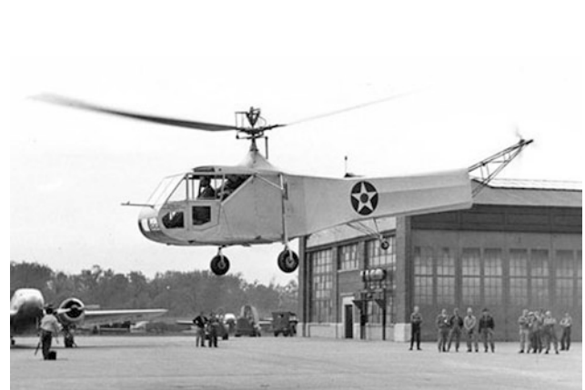
Fig. 2.15 Production version of Sikorsky S-47/R-4 in operation (1941), (Credit Igor I. Sikorsky Archives)
