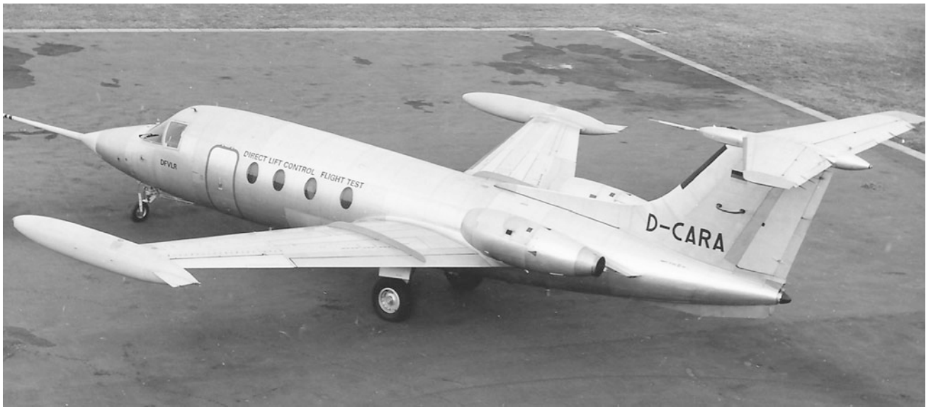
Fig. 7.28 HFB 320 ready for DLC flight tests (1972/73)
