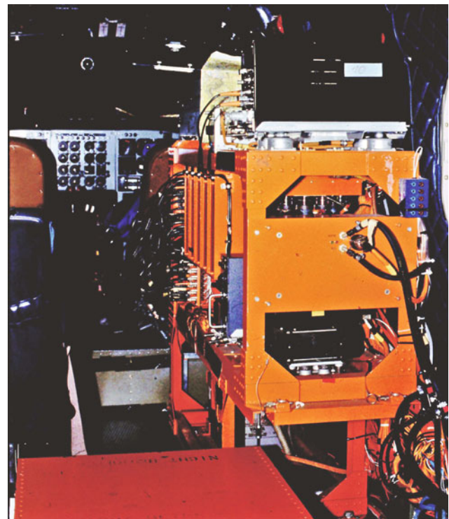
Fig. 6.115 Signal processing in the TNT test aircraft (Credit Bernd Krag)
