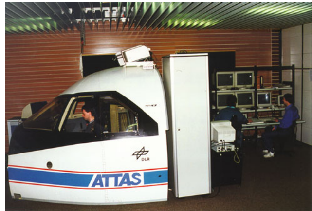
Fig. 9.36 ATTAS simulation cockpit (external view)
