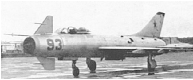
Fig. 6.60 Sukhoi L02-10 with two additional vertical control surfaces
