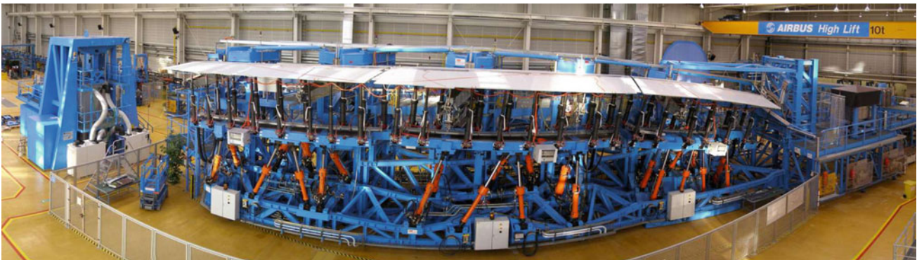
Fig. 6.149 Wing system test bench
