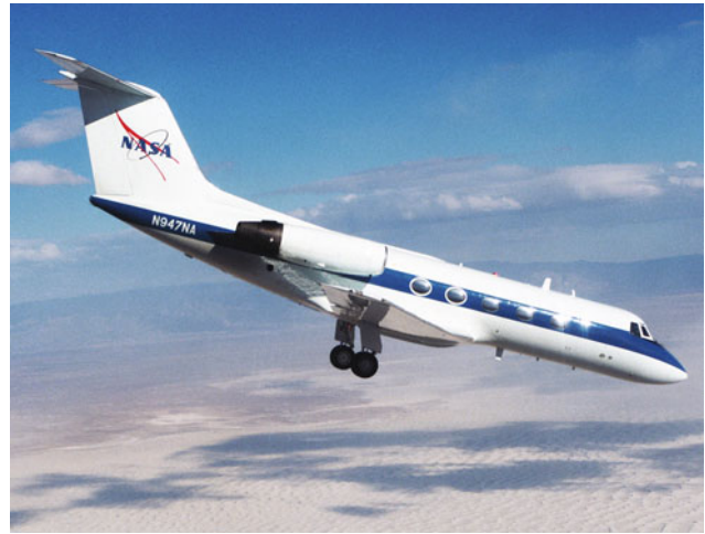
Fig. 5.55 STA Shuttle approach simulation
