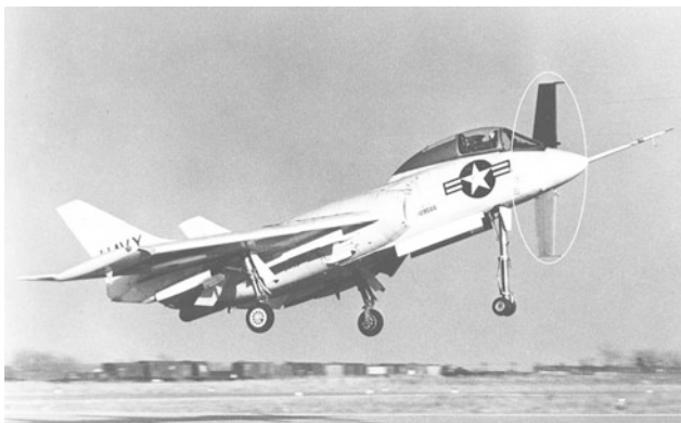
Fig. 5.15 F7U-3 with additional control surfaces
