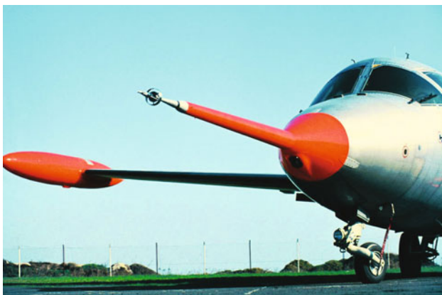
Fig. 7.22 Noseboom with Dornier flight log
