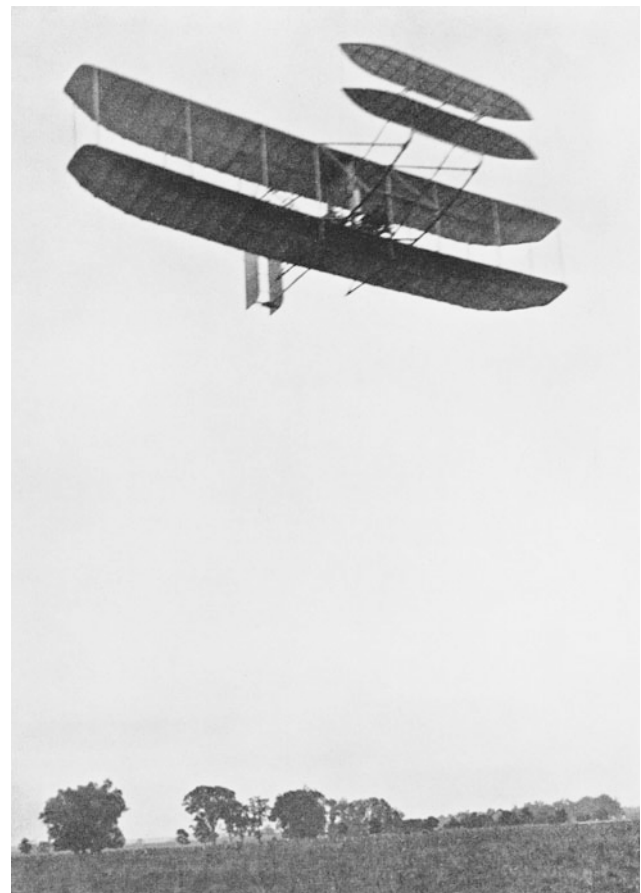
Fig. 2.2 The first fully controllable aircraft, the “Flyer III” in flight (1905), (Credit Deutsches Museum)
