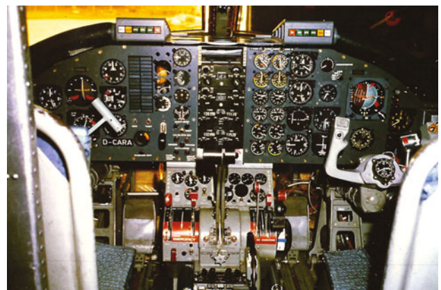
Fig. 7.18 Instrument panel and test pilot station on the right with primary flight display
