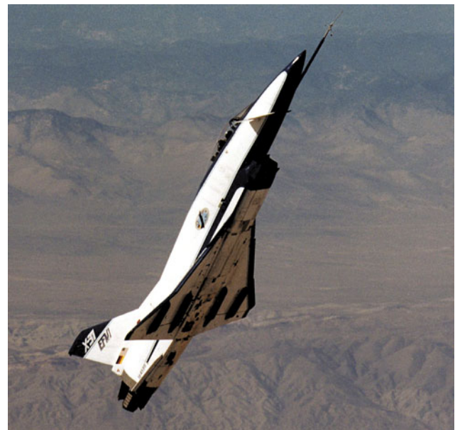
Fig. 6.130 X-31A EFM post-stall demonstration
