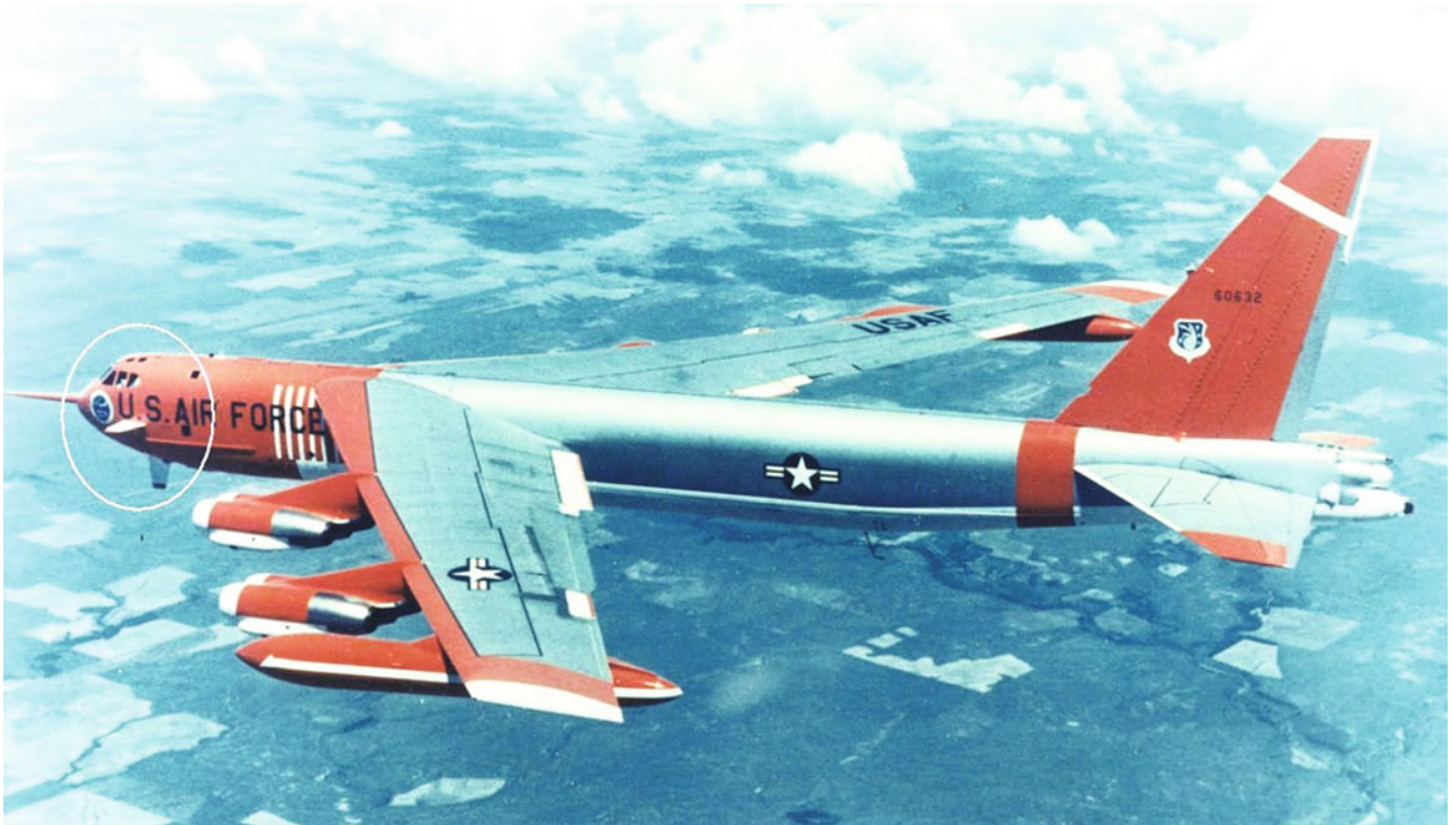
Fig. 6.32 Boeing NB-52E CCV (AF 56-0632) with canard control surface triple
