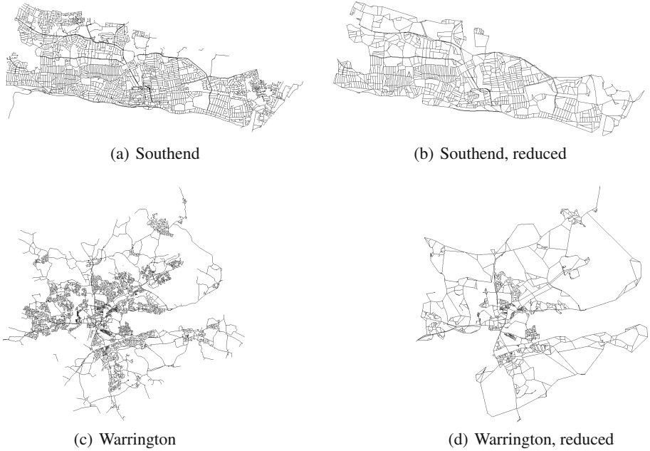
Fig. 7. Original maps and reduced graphs for Southend and Warrington road networks, illustrating grid-like and tree-like road networks.
