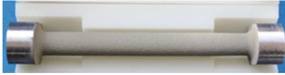
Fig. 2 The general view of tensile samples before mechanical test
