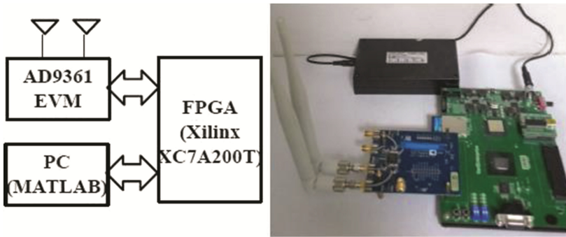
Fig. 6. Software defined radio platform with AD9361 EVM and Xilinx/SMIMS AC701 evaluation board
