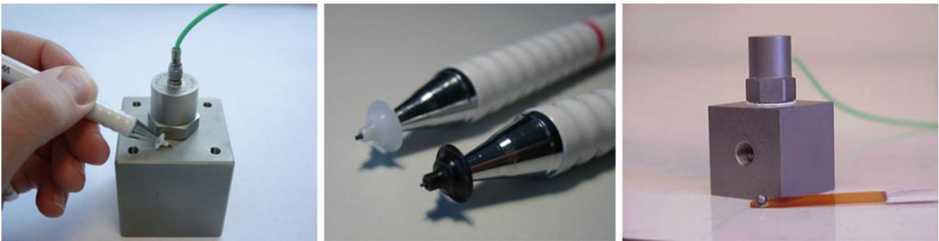
Fig. 5.7 Pencil lead break, or impact with a steel ball on a steel cube of 25.4 \text{ mm}^3 (The pencil is using a cushion tube at the tip to prevent multiple impacts, similar to the HSU-Nielson source for acoustic emission testing)
