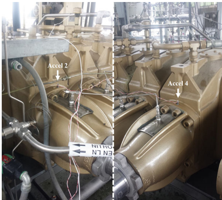
Fig. 7.3 Close-up view of accelerometers 2 and 4
