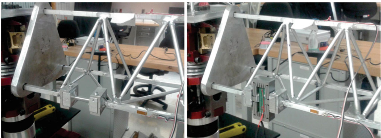
Fig. 14.7 PZT stack actuator and two strain gauge on crane structure
