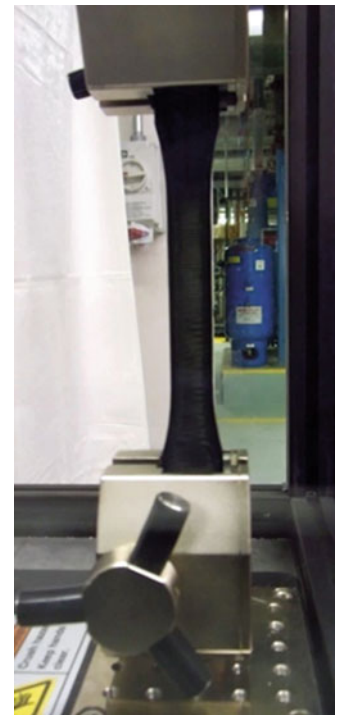
Fig. 13.2 Testing to determine the temperature coefficient: (a) Industry standard strain gauge ( left ) and an additive manufactured U-Gage ( right ), (b) Experimental setup for the temperature coefficient tests
