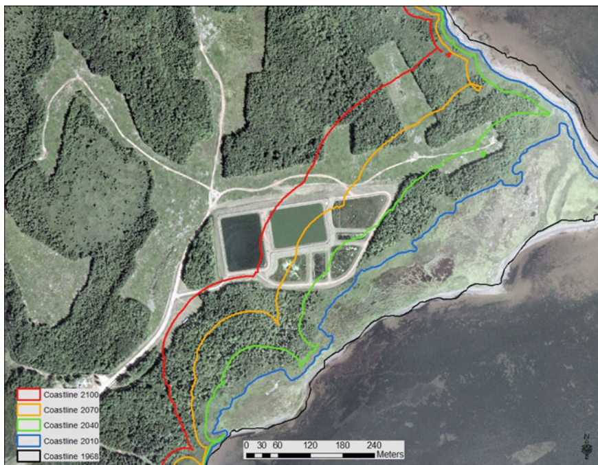
Fig. 14.2 Settling Ponds on Lennox Island depicting areas at high, medium, and low risk to coastline recession. Background image is 2010 Prince Edward Island orthophoto (own figure)
