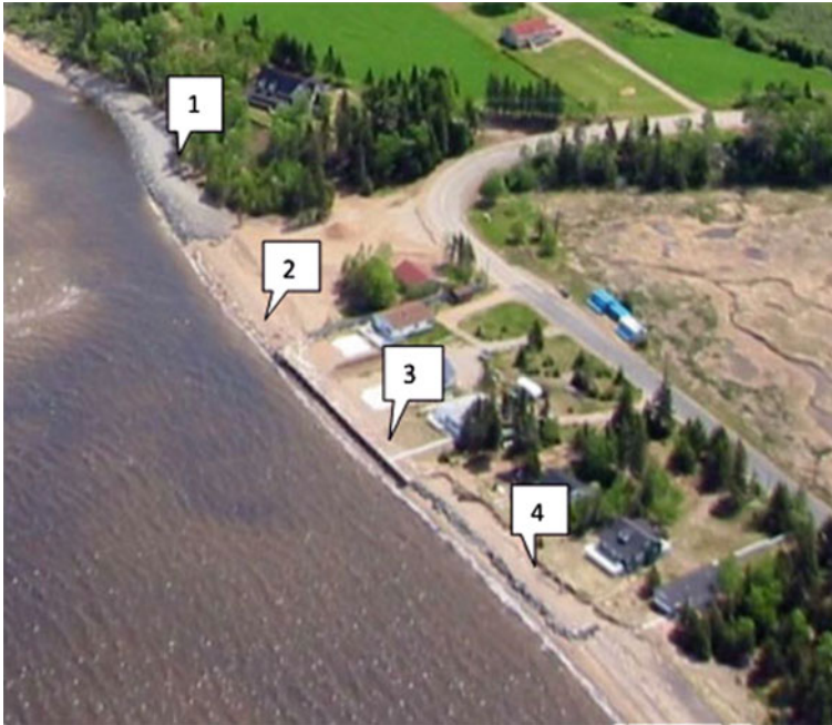
Fig. 5.3 Different types of protection structures at Pointe-Carron: 1 heavy shale riff-raff, 2 light rock riff-raff, 3 cement wall, 4 large rock riff-raff. Source Chouinard et al. (2009)
