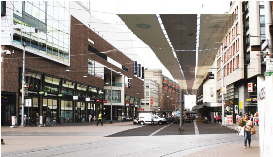
Fig. 20.5 The Grotemarktstraat in The Hague with canvas sheets to improve thermal comfort on hot days
