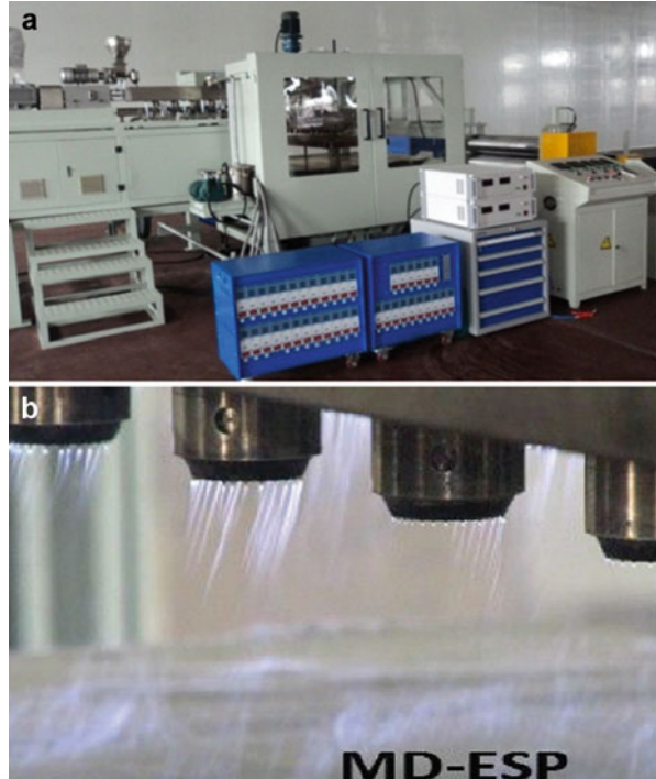
Fig. 16 Photo of (a) the pilot prototype of the polymer melt differential electrospinning device. (b) Pilot prototype in running
