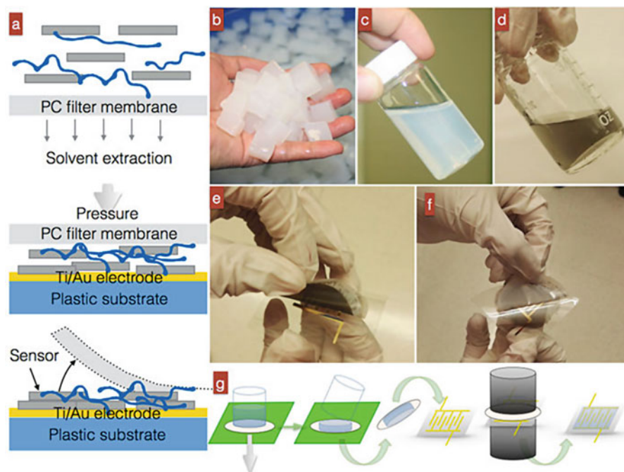
Fig. 9 Fabrication of alcohol-sensing device based on graphene nanosheets (Gr) and bacterial cellulose nanofibers (BC): (a) Gr/BC sensors are fabricated by vacuum filtration. (b) The BC hydrogels at 0.5 wt%. (c) The extraction process of 1 wt% aqueous suspension in BC after TEMPO treatment. (d) Gr/BC colloidal mixture with 40 wt%Gr volume. (e) At 40 wt% Gr wet base load Gr/BC device delamination sputtered Ti/Au electrode interdigital on a plastic substrate. (f) The process stripped the substrate from dry Gr/BC vacuum compression/drying at 60 °C. (g) The whole process of equipment assembly [48]. (Copyright 2017, Nature)
