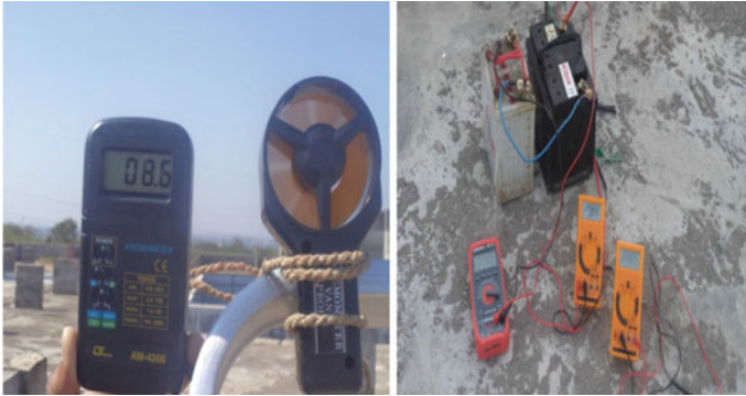
Fig. 9 Wind speed measurement on Anemometer
