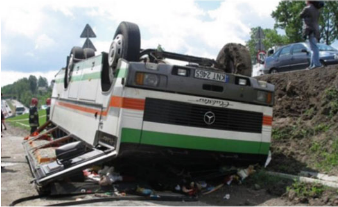
Fig. 1 Damaged structure of bus in the case of rollover [1]
