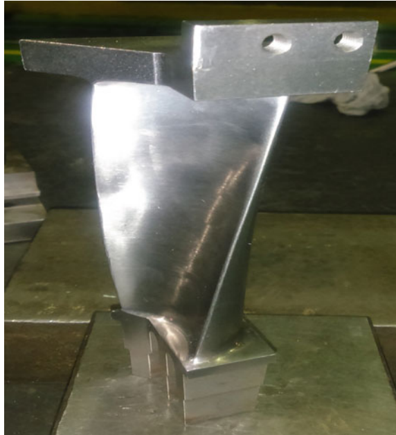
Fig. 1 View illustrating blade with rhombic shaped shrouds
