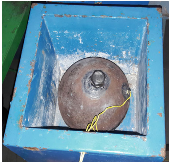
Fig. 2 Spherical capsule in TES tank
