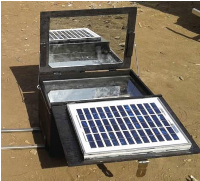
Fig. 2 Fabrication assembly of solar dryer
