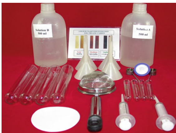
Fig. 1 Different components of soil organic carbon detection kit
