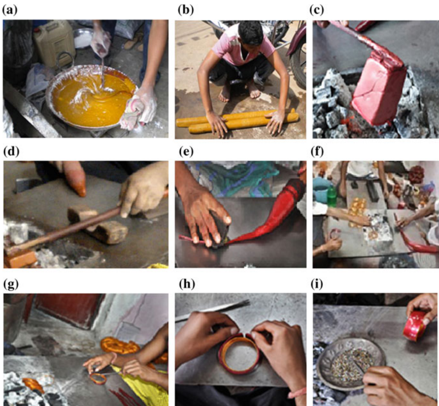
Fig. 1 a Melting of Lac pieces ( in Kadai ), b Rolling of Lac as rods, c Heating the uncolored lac, d Rubbing colored Lac, e Coil formation using hattha , f Heating the coil, g Shaping the coil, h Putting the metal bangles, i Fixing the colored stones into coil into bangles
