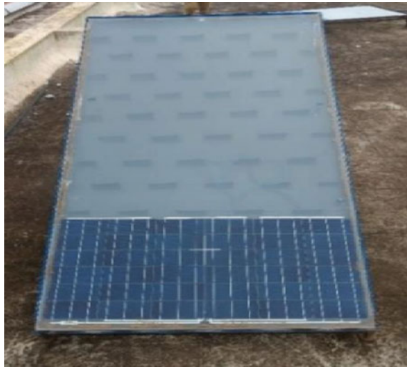
Fig. 2 Experimental set-up of solar air heater
