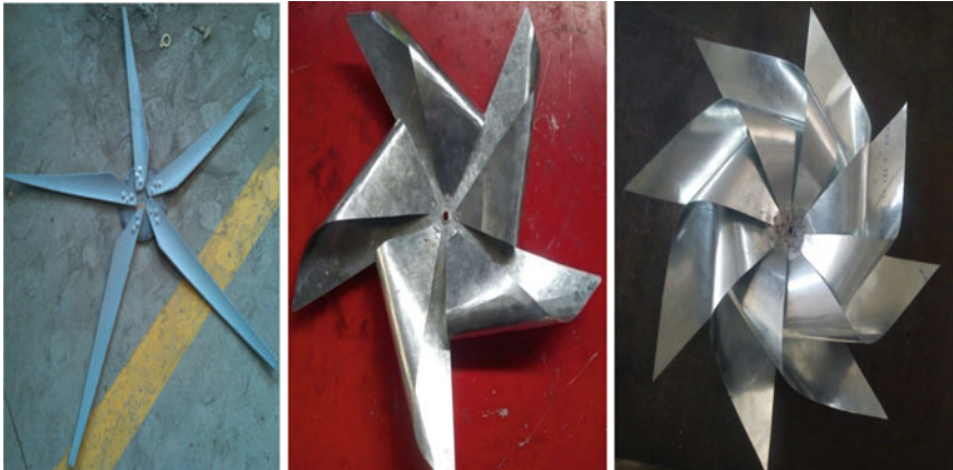
Fig. 2 PVC and sheet metal model of five and eight blades
