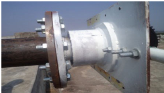
Fig. 5 Nacelle bed plate with yawing assembly
