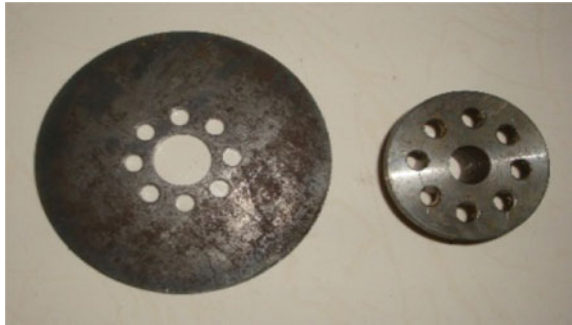
Fig. 4 Rotor hub plate and bush
