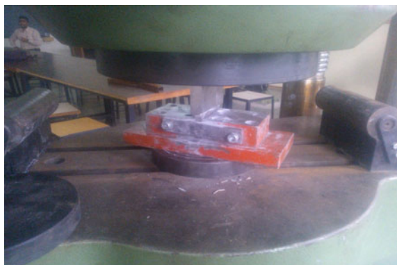
Fig. 2 Die compacting for tensile and impact test specimen
