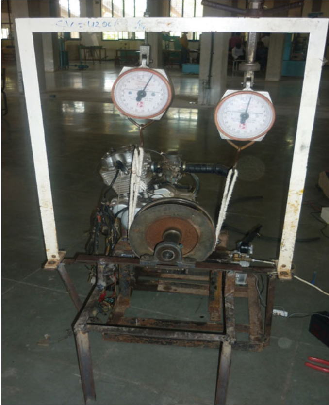
Fig. 2 Pictorial view of dynamometer
