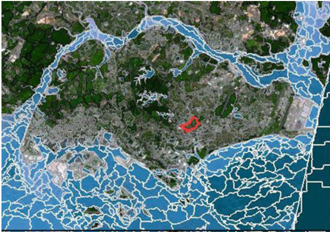
Fig. 4 Classified image of water (using eCognition)
