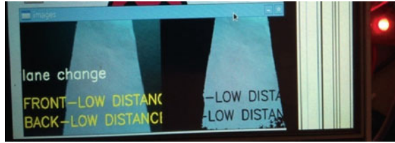
Fig. 11 Output when lane, front side, and back side obstacle is detected
