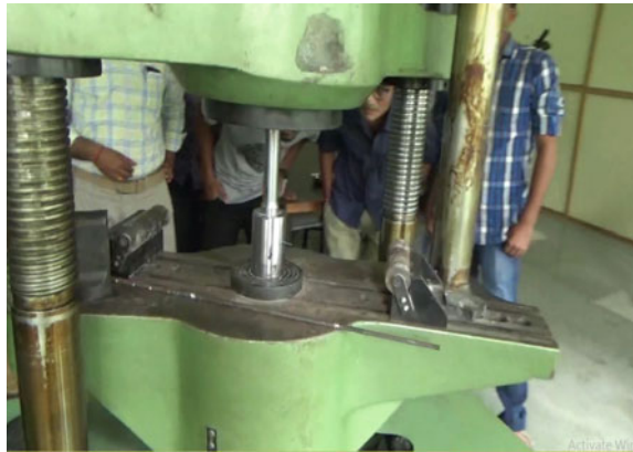
Fig. 3 Die compacting for lateral compression test specimen
