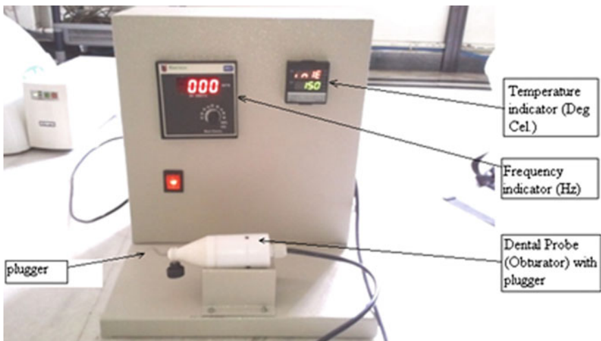
Fig. 5 Device based on a new method of ‘heat vibration and compaction’ used to perform obturation
