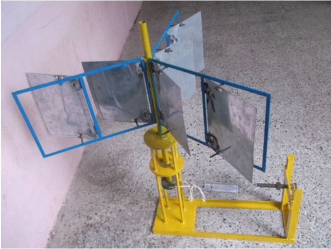
Fig. 1 Photograph of shutter type vertical axis wind turbine (STVAWT)
