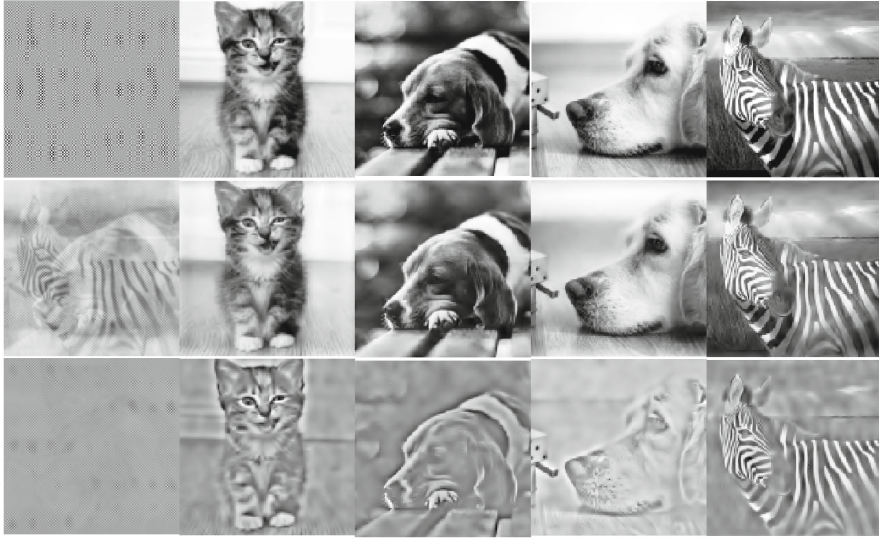
Fig. 3. First row: illustration of \mathbf{O}_1 , then the four initial sources. Second row: illustration of \mathbf{X}_1 for m = 34 and \frac{\|\mathbf{O}\|_\infty}{\|\mathbf{AS}\|_\infty} = 1 and then the sources estimated with rGMCA. Third row: illustration of \mathbf{X}_1 for m = 20 and \frac{\|\mathbf{O}\|_\infty}{\|\mathbf{AS}\|_\infty} = 10 and then sources estimated with PCP+GMCA. The sources were estimated for m = 34 and \frac{\|\mathbf{O}\|_\infty}{\|\mathbf{AS}\|_\infty} = 1 .
