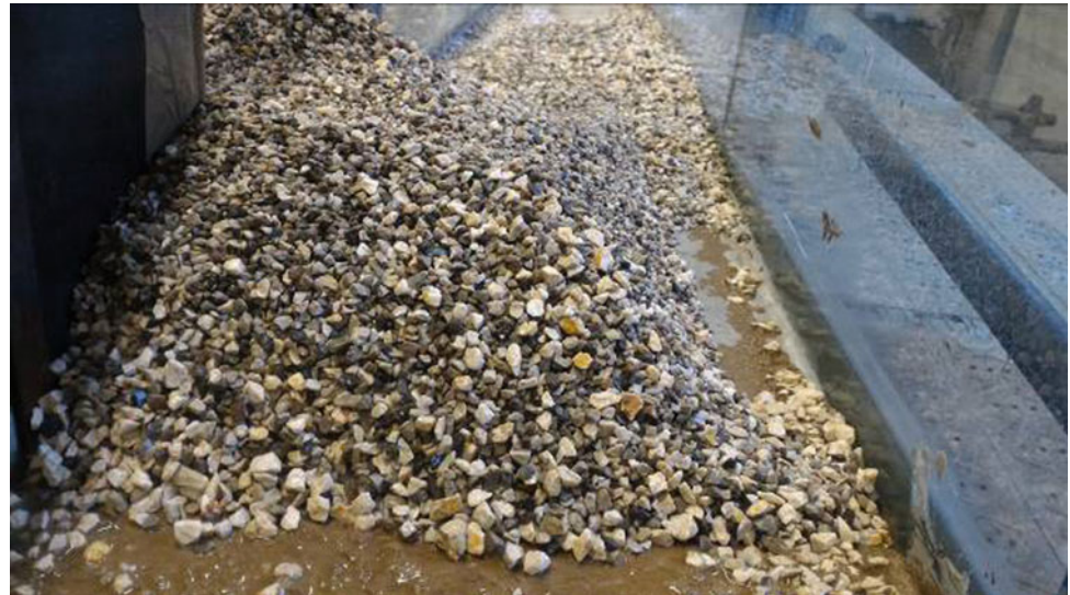
Fig. 3 Example (run 9) of the partial blockage of the main channel caused by the debouch of a stony debris flow generated along the tributary channel
