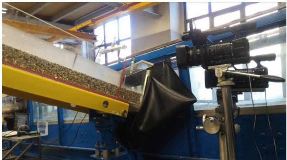
Fig. 2 Experimental apparatus consisting in a lateral tributary flume connected to a downstream main channel
