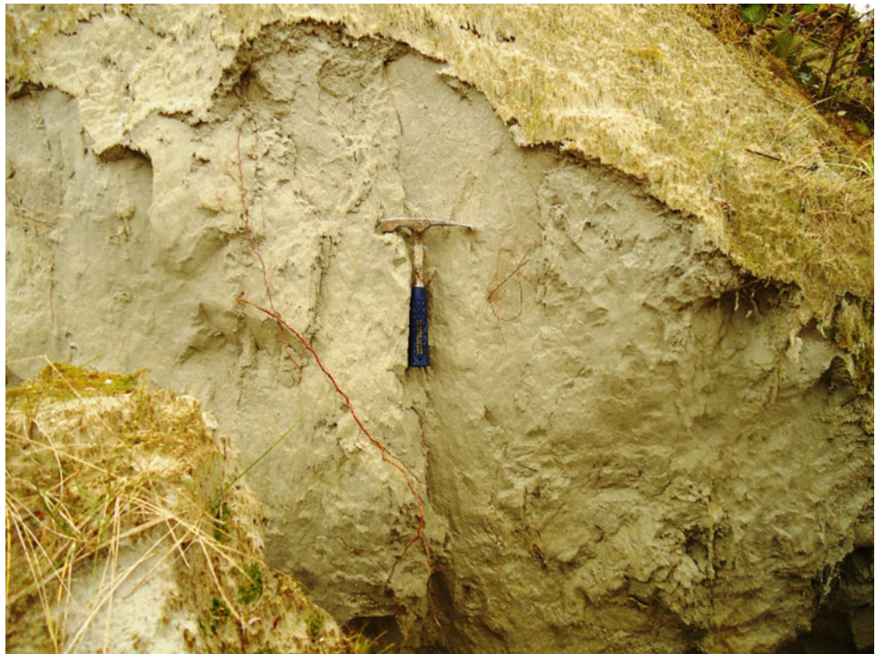
Fig. 3 Volcanic tuff materials within landslide blocks at the collapse zone of the Aratozawa landslide
