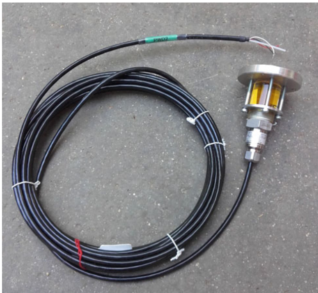
Fig. 6 Pore water pressure sensor with an oil-filled reservoir
