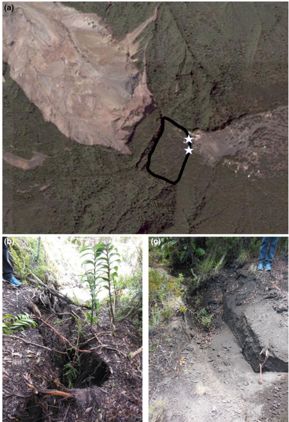
Fig. 4 a Continuous line bounds the triggering area of the potential landslide with volume equal to 3.5 \times 10^6 \text{ m}^3 (Background image from Google Earth); star symbols indicate the position of the b and c details of the existing open deep fissure
