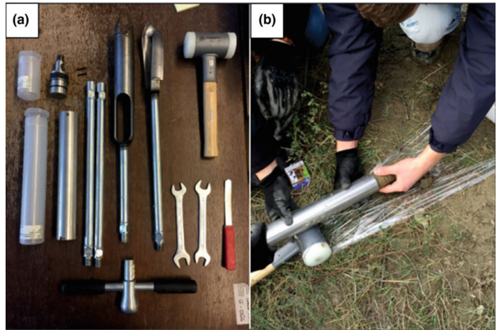
Fig. 4 Eijkelkamp sampling tool applied to the soil sampling in the Vinodol Valley: a manual drilling equipment; b field soil sampling
