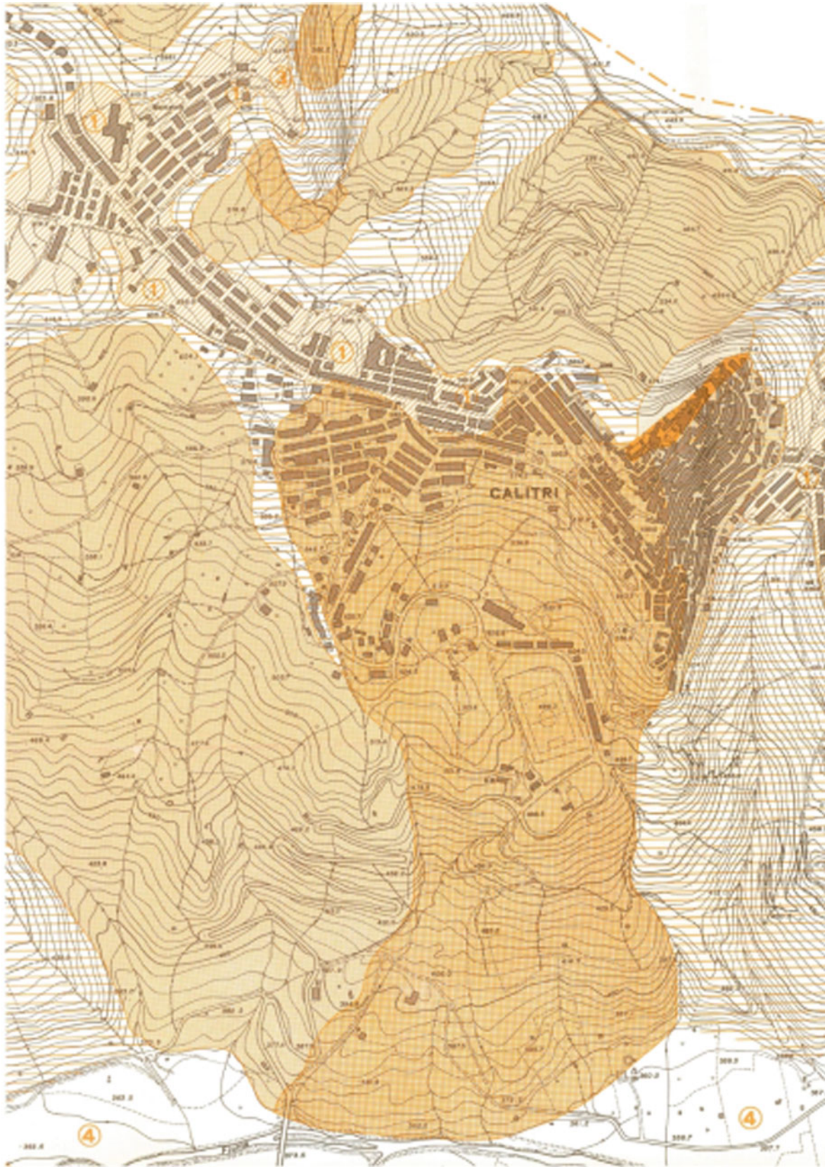
Fig. 3 The original map drawn by Samuelli-Ferretti and Siro (1983a) for the PFG-CNR microzonation of Calitri after the 1980 earthquake
