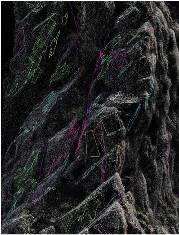
Fig. 3 Automatically generated patches plotted on the point cloud in Split-FX software
