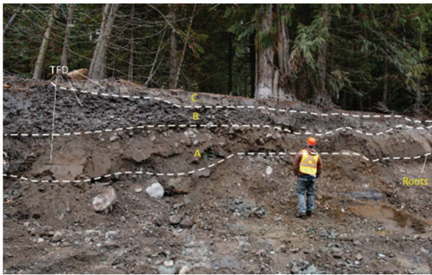
Fig. 2 Flow deposits at the pre-event Hazeltime Creek channel. Pre-event surface identified by the presence of roots ( middle right ). TFD Tailings flow deposit. A Red layer of sandy tailings. Likely initial stages of the flow where water content is assumed to be higher than solids. B Mix of tailings and native material entrained from channel bed and banks. C Silty-clay deposits ( Photo by ARCHER 2015 )
