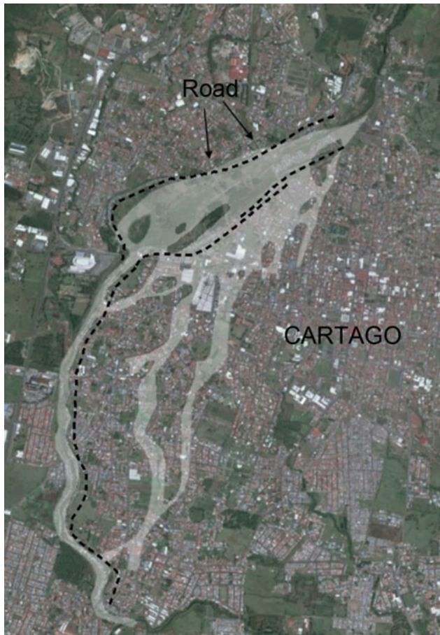
Fig. 3 Dot lines are the levees that were built after the 1963–1965 events. Arrows indicate the position where the roads cut the levees to cross the area. The grey shadowed area is the main deposit of the debris flow occurred on December 9, 1963
