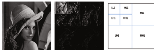
Fig. 5. Representation of a wavelet transform of the Lena image at 2 levels
