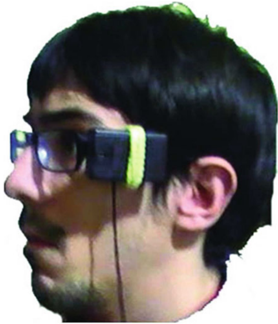
Fig. 6 Accelerometer-based sensor node attached on the head [6]
