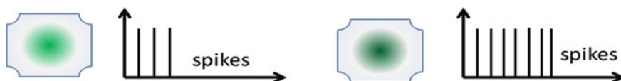
Fig. 10 Spiking behaviour of TO-neurons: left low power of neuron’s activity, right high power of neuron’s activity
