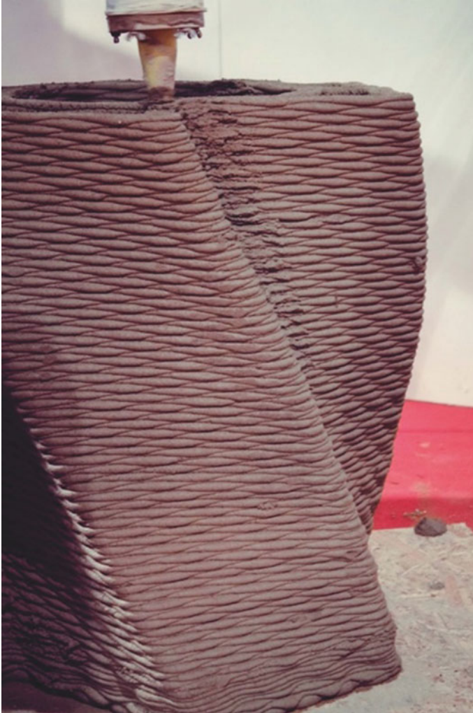
Fig. 3 The 3D printing of a cement-based full scale column has been tested to understand the potential of a Delta with a height of 4 m (ACTLAB, ABC Dept., Politecnico di Milano)
