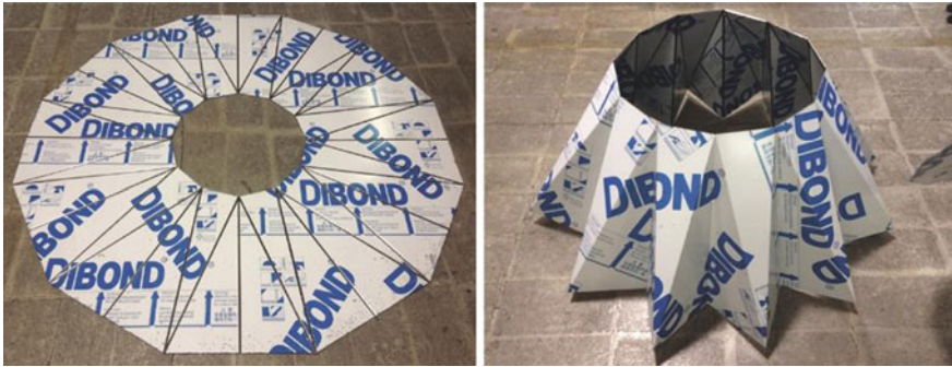
Fig. 4 Dot & Line : Cutting pattern (left) and folded structure from ACM board (right)
