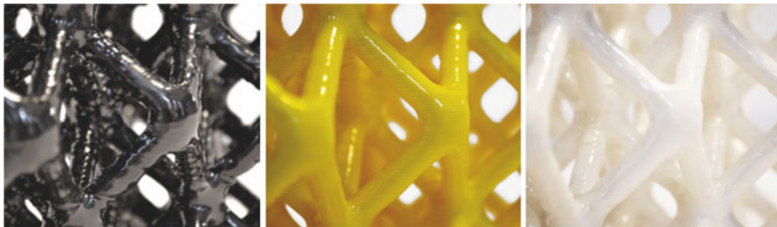
Fig. 6 Material research, carried out by the composite thermoplastic tests with maximum performance, and post-production, using epoxy resin impregnation. (From left) Polylactic Acid, acrylonitrile styrene acrylate (ASA) and Polycarbonate (ACTLAB, Politecnico di Milano)
