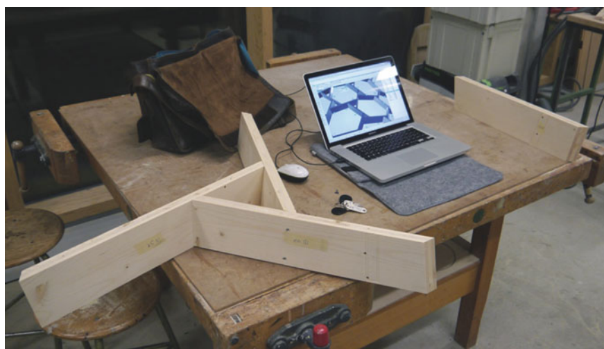
Fig. 8 Testing the first reciprocal knot
