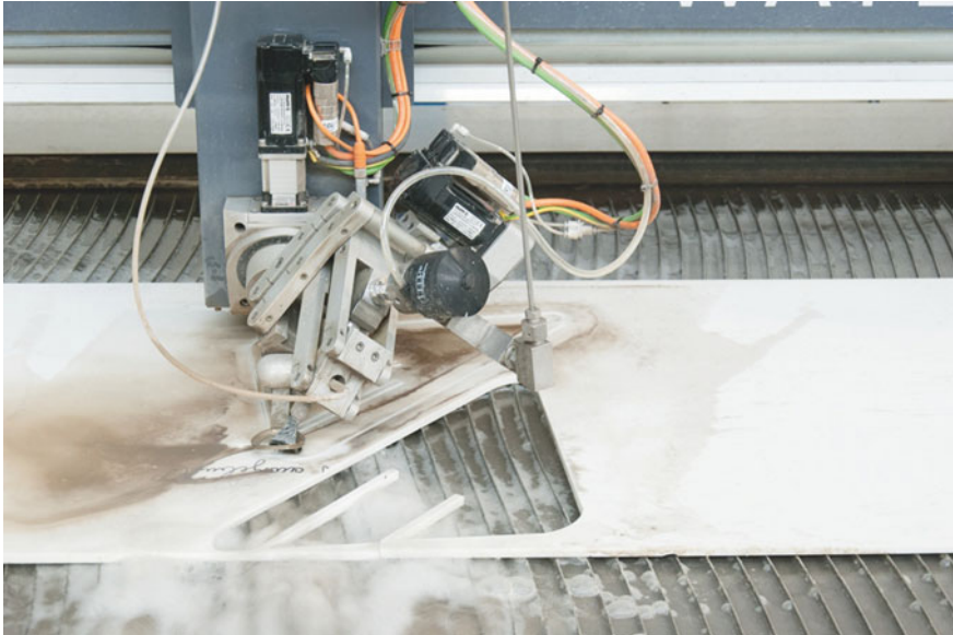
Fig. 5 Cutting the composite panels with a WaterJet
