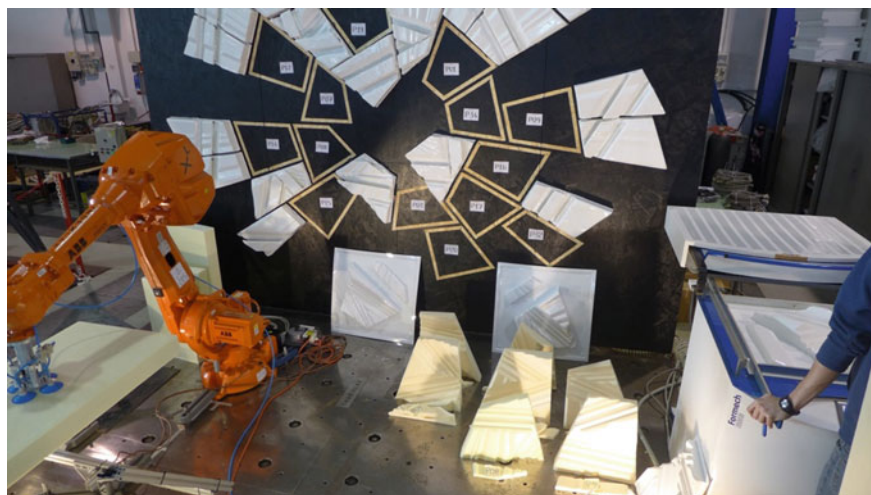
Fig. 7 Robotic hot-wire cutting and thermoforming. Indexlab 2014, Politecnico di Milano
