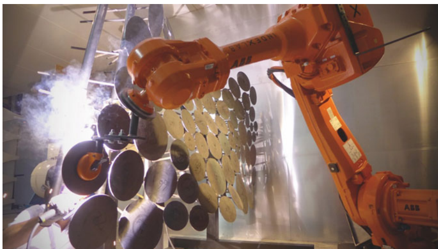
Fig. 4 Circle packing. Robotic pick and place and adaptive welding. Indexlab 2013, Politecnico di Milano, Nieder
