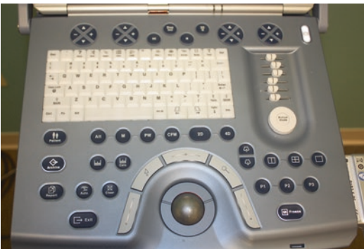
Fig. 4.7 The dominant hand generally operated the console. Unlike the BK console, (BK Ultrasound, Analogic, Peabody, MA, USA), the GE Voluson e buttons on the console (GE Healthcare, Chicago, IL, USA) are multi-functional; their function corresponds to the menu at the bottom of the screen. © Shobeiri 2013
